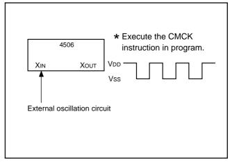
Fig. 45 External clock input circuit
