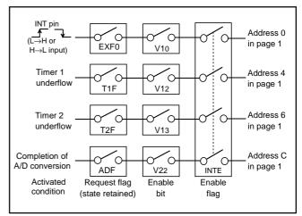
Fig. 15 Interrupt system diagram
