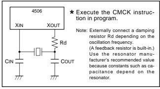
Fig. 43 Ceramic resonator external circuit
