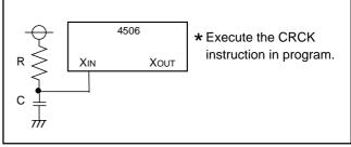
Fig. 44 External RC oscillation circuit
