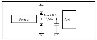
Fig. 52 Analog input external circuit example-2
