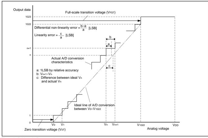
Fig. 32 Definition of A/D conversion accuracy
