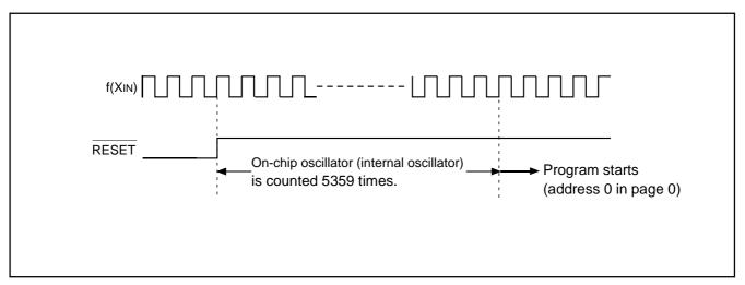
Fig. 33 Reset release timing
