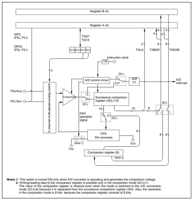
Fig. 28 A/D conversion circuit structure
