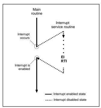
Fig. 13 Program example of interrupt processing
