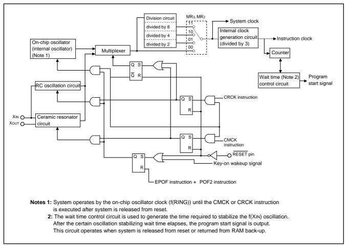
Fig. 40 Clock control circuit structure
