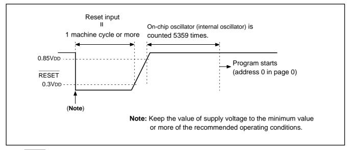
Fig. 34 RESET pin input waveform and reset operation
