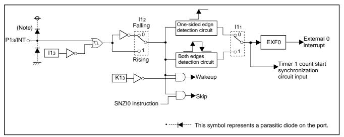
Fig. 17 External interrupt circuit structure
