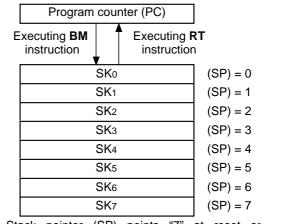
Stack pointer (SP) points "7" at reset or returning from RAM back-up mode. It points "0" by executing the first BM instruction, and the contents of program counter is stored in SKo. When the BM instruction is executed after eight stack registers are used ((SP) = 7), (SP) = 0 and the contents of SKo is destroyed.
