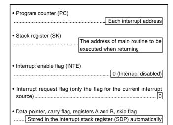
Fig. 14 Internal state when interrupt occurs
