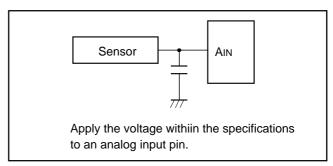
Fig. 51 Analog input external circuit example-1
