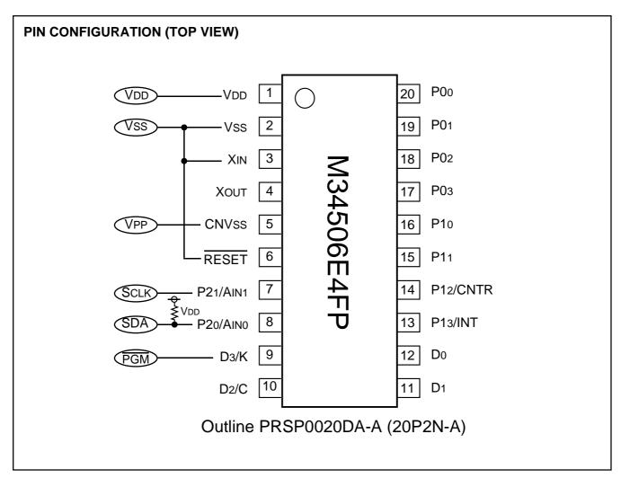
Fig. 54 Pin configuration of built-in PROM version
