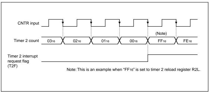
Fig. 23 Count timing diagram at CNTR input
