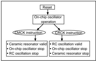
Fig. 41 Switch to ceramic resonance/RC oscillation
