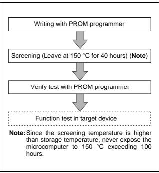
Fig. 53 Flow of writing and test of the product shipped in blank
