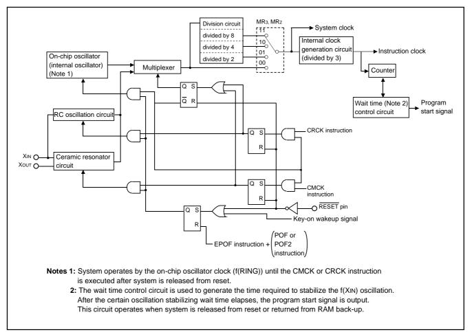
Fig. 42 Clock control circuit structure
