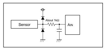
Fig. 54 Analog input external circuit example-2
