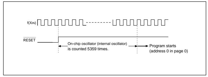
Fig. 33 Reset release timing
