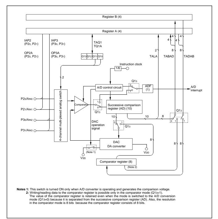
Fig. 28 A/D conversion circuit structure
