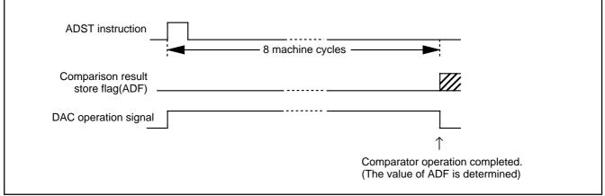
Fig. 31 Comparator operation timing chart
