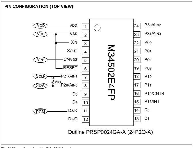
Fig. 56 Pin configuration of built-in PROM version
