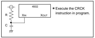
Fig. 46 External RC oscillation circuit
