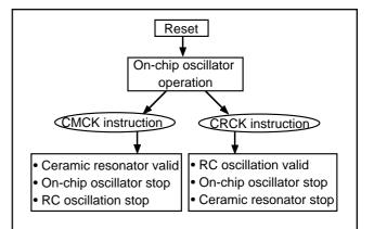
Fig. 43 Switch to ceramic resonance/RC oscillation
