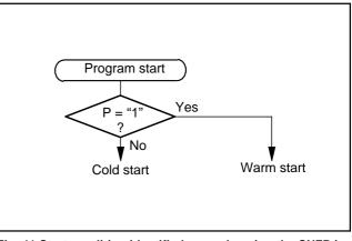
Fig. 41 Start condition identified example using the SNZP instruction
