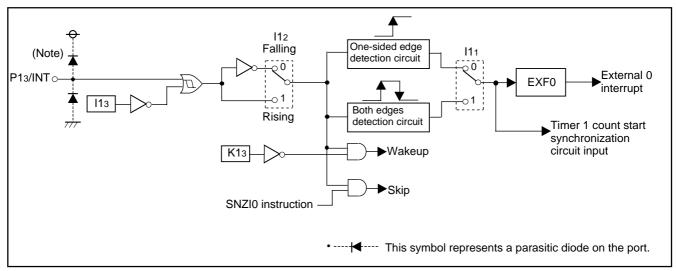
Fig. 17 External interrupt circuit structure
