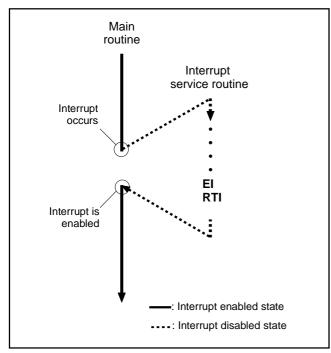
Fig. 13 Program example of interrupt processing
