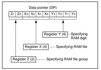
Fig. 8 Data pointer (DP) structure
