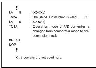
Fig. 52 A/D conversion interrupt program example
