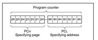
Fig. 7 Program counter (PC) structure
