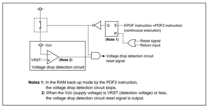
Fig. 37 Voltage drop detection circuit
