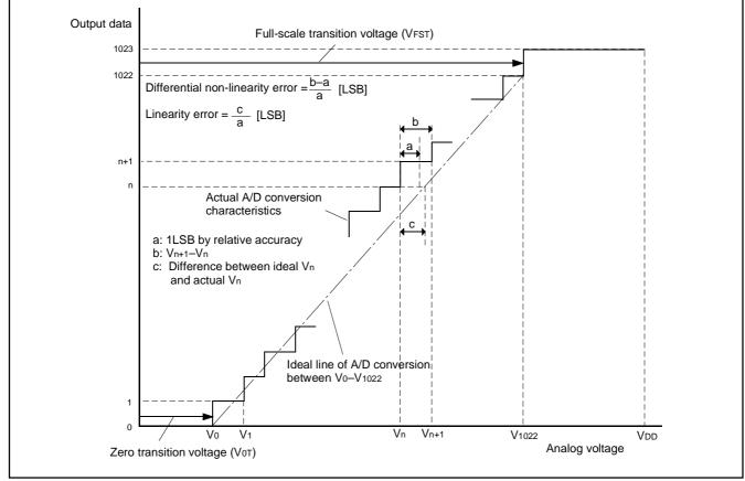
Fig. 32 Definition of A/D conversion accuracy
