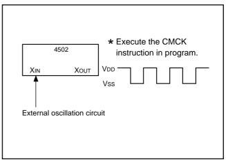
Fig. 47 External clock input circuit
