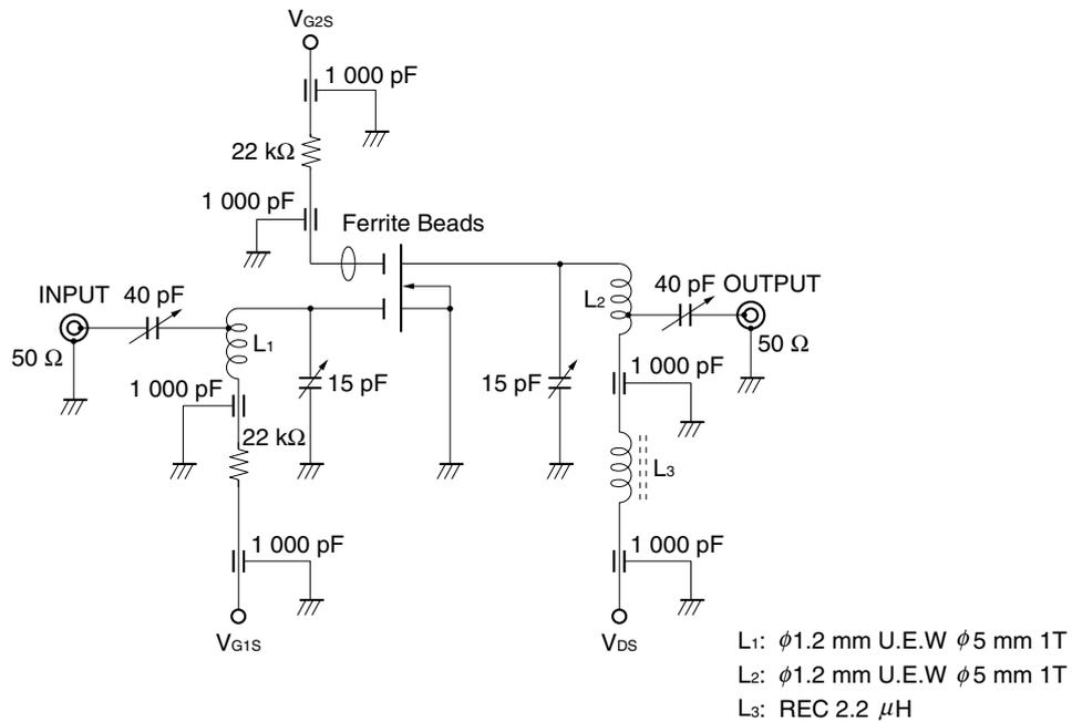
**NF TEST CIRCUIT AT  $f = 55 \text{ MHz}$**
