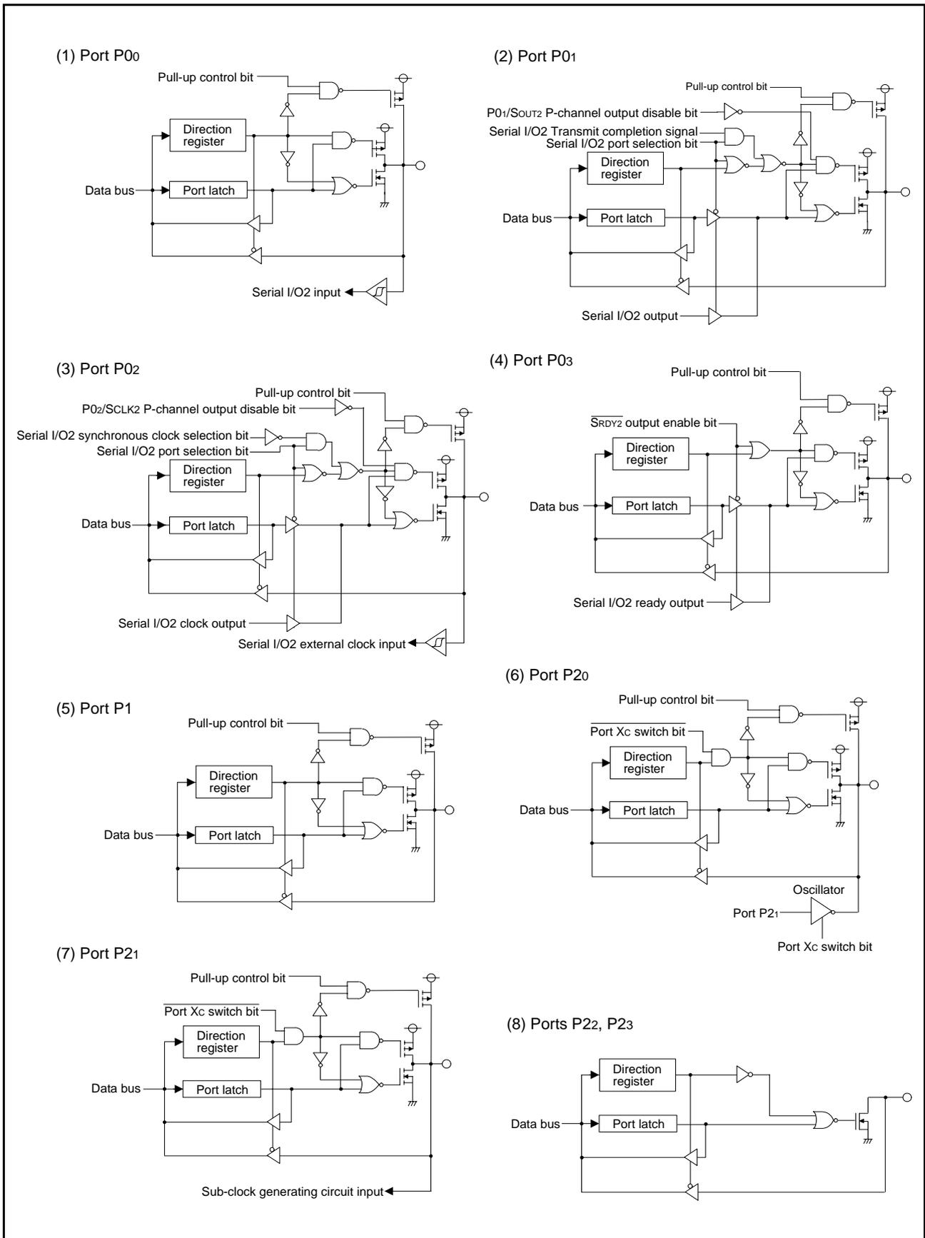
Fig 10. Port block diagram (1)
