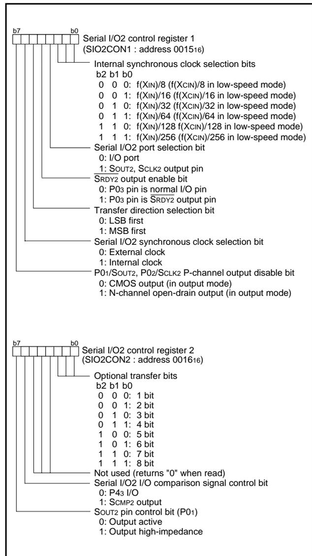
Fig 25. Structure of Serial I/O2 control registers 1, 2
