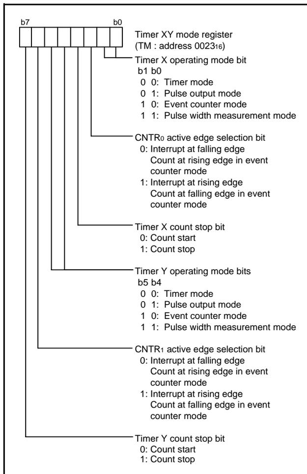
Fig 17. Structure of timer XY mode register
