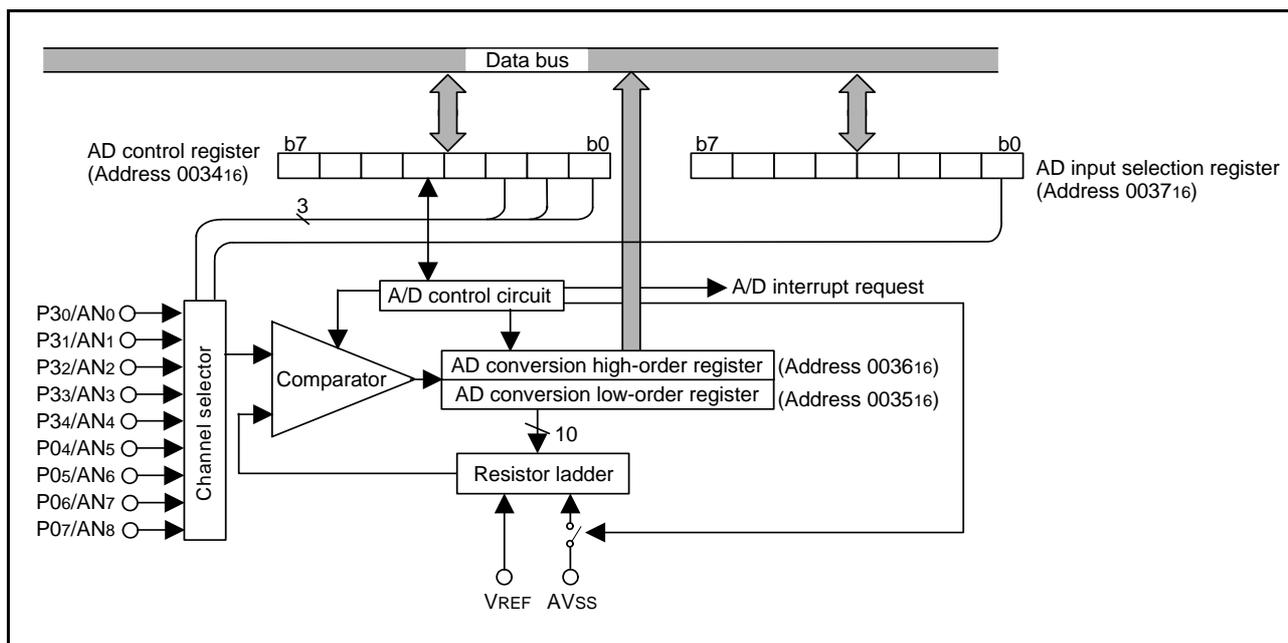
Fig 36. Block diagram of A/D converter
