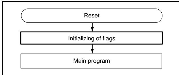
Fig 49. Initialization of processor status register
