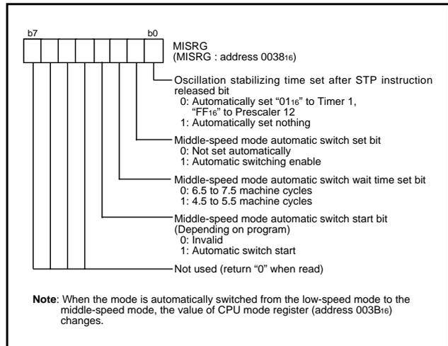
Fig 44. Structure of MISRG
