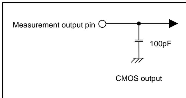
Fig 47. Circuit for measuring output switching characteristics
