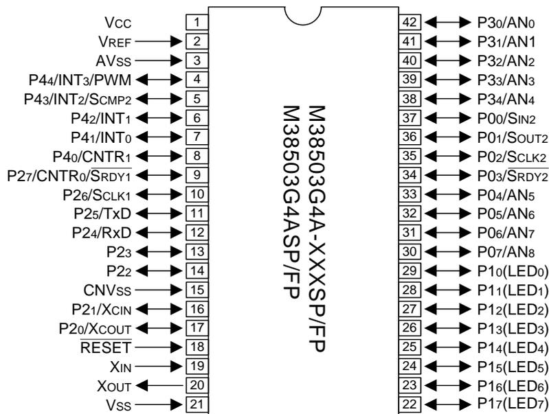
Package type : SP ..... PRDP0042BA-A (42P4B) (42-pin shrink plastic-molded SDIP)
