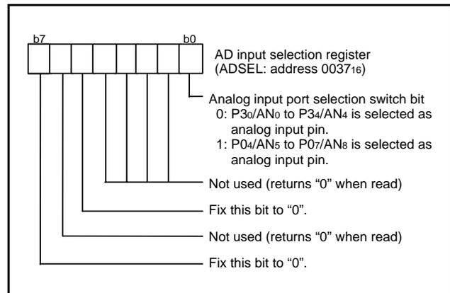
Fig 34. Structure of AD input selection register
