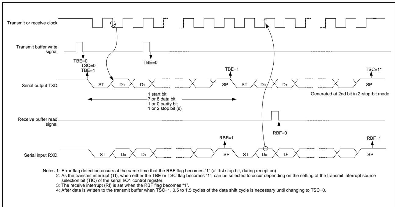
Fig 23. Operation of UART serial I/O1 function
