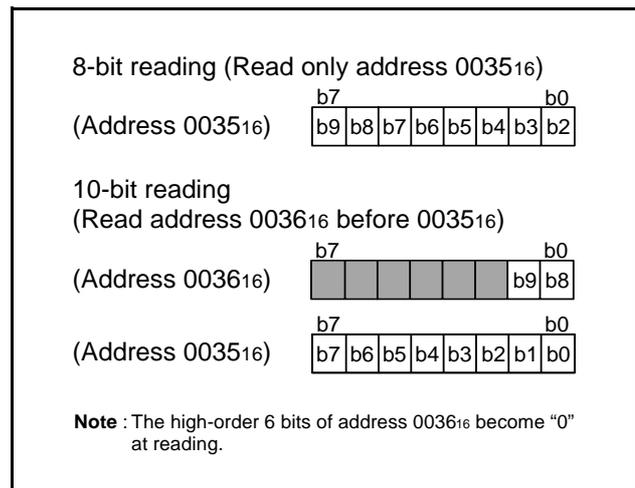
Fig 35. Structure of AD conversion registers
