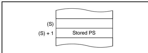
Fig 50. Stack memory contents after PHP instruction execution
