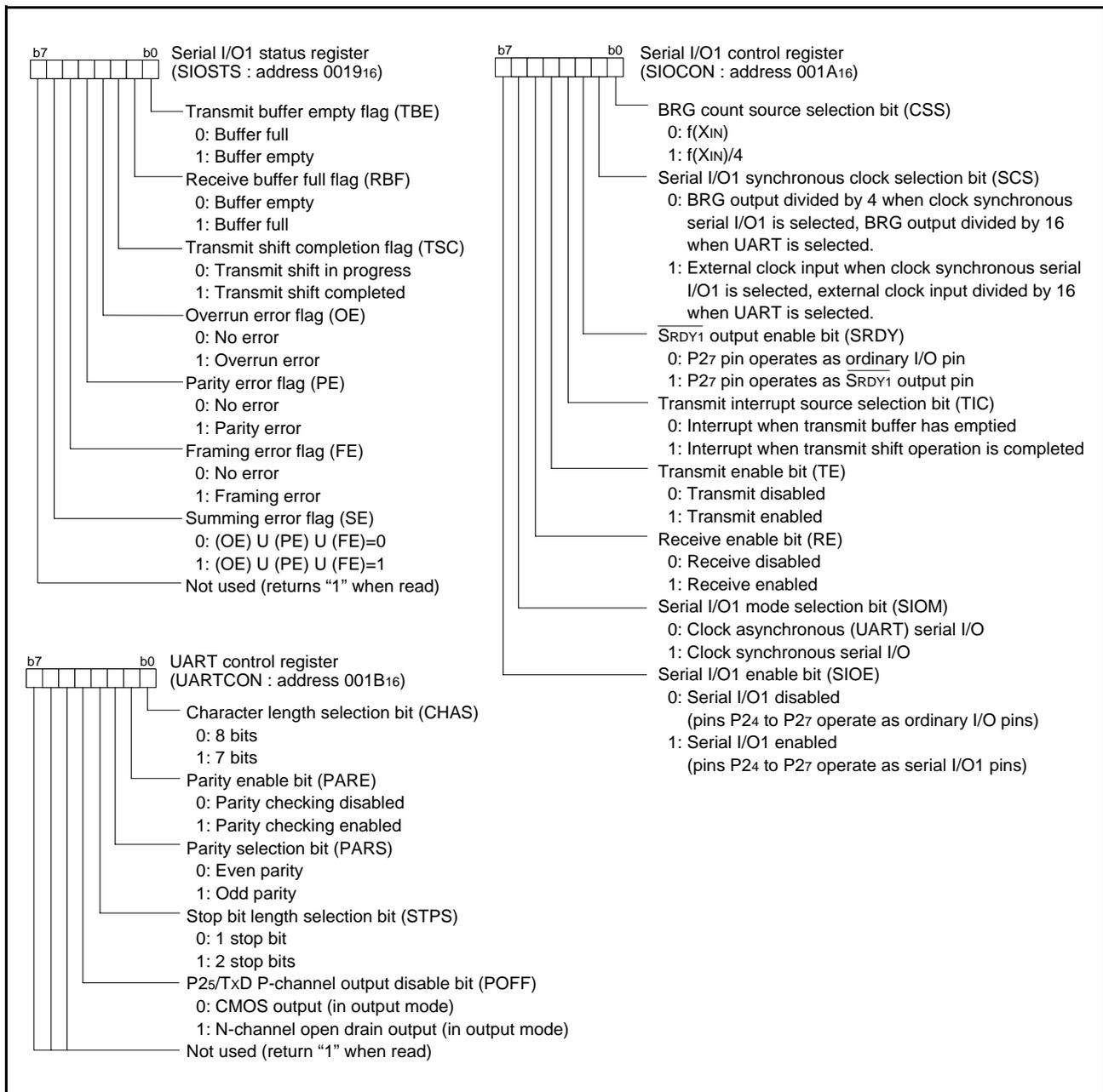
Fig 24. Structure of serial I/O1 control registers
