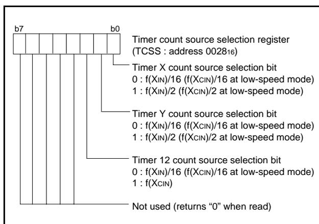
Fig 18. Structure of timer count source selection register
