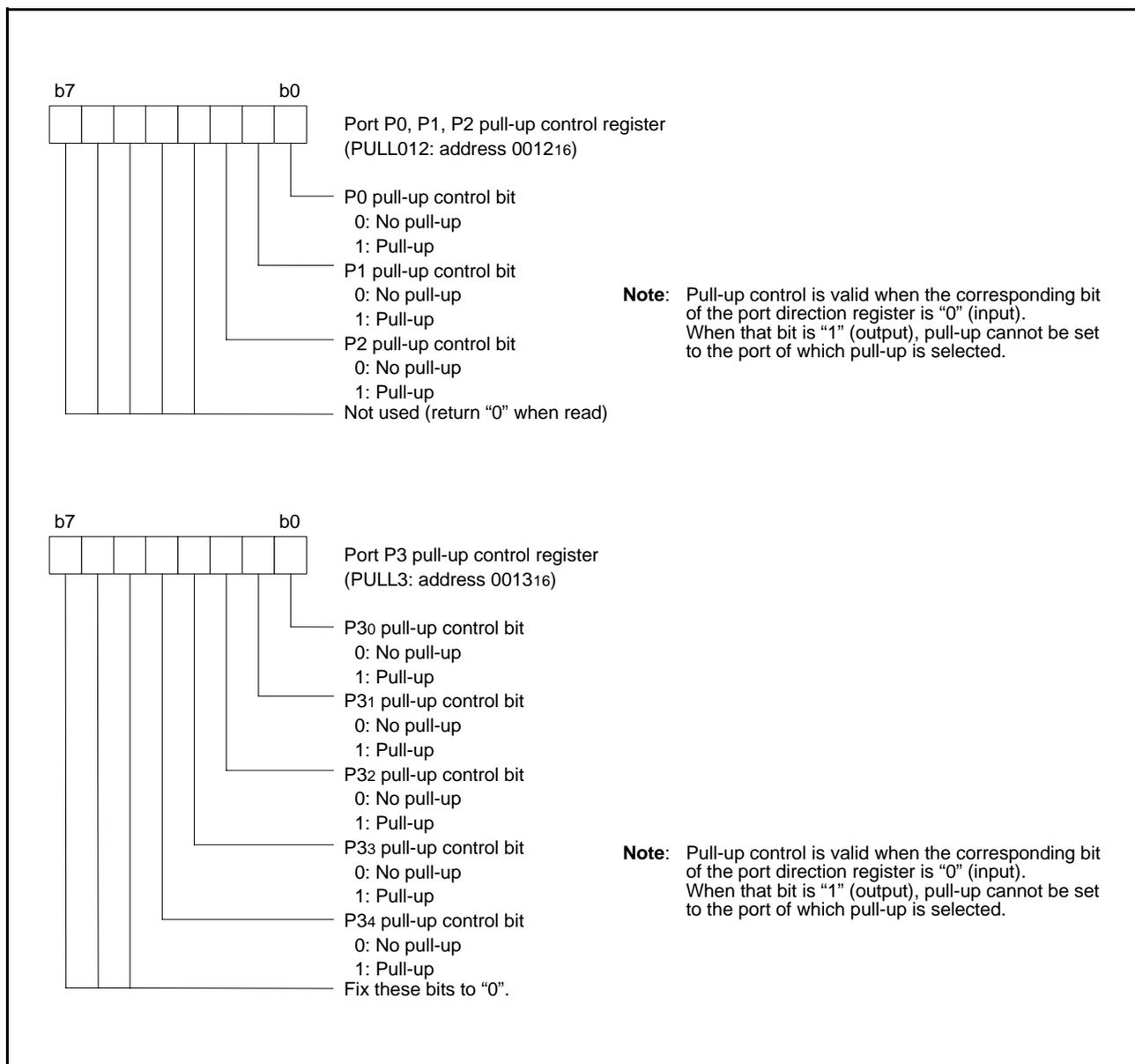
Fig 13. Structure of port registers (1)
