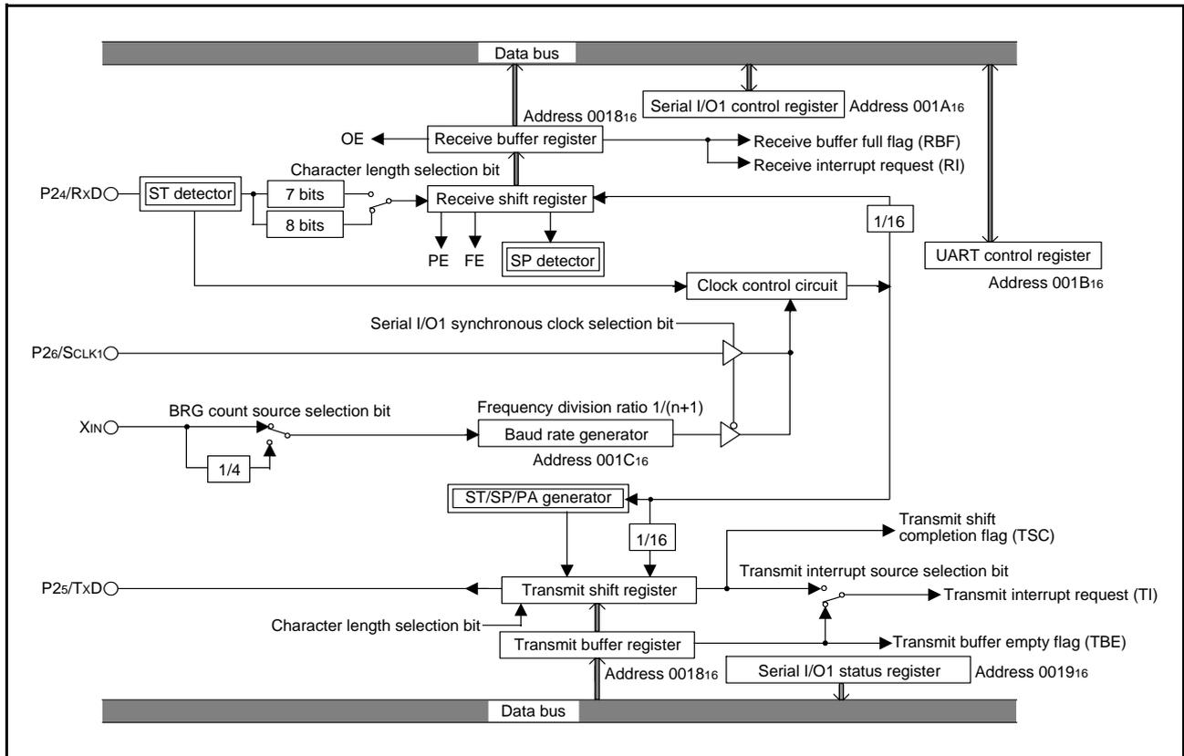
Fig 22. Block diagram of UART serial I/O1
