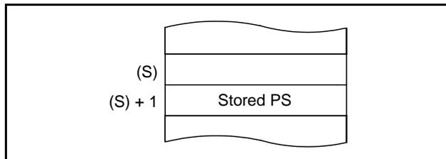
**Fig 88. Stack memory contents after PHP instruction execution**
