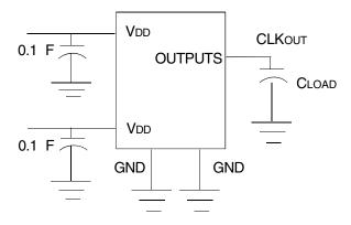
Test Circuit for All Parameters
