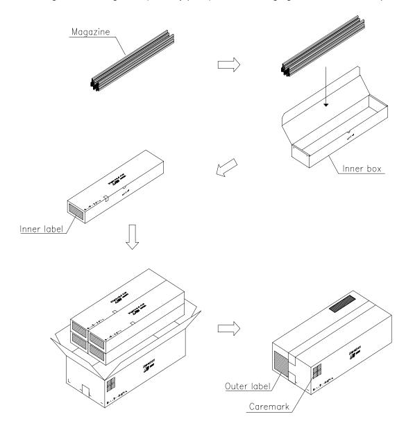
\* Packing form for magazine (Non dry pack). The following figure shows an example.
