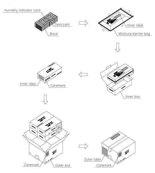
\* Packing form for tray (Dry pack). The following figure shows an example.
