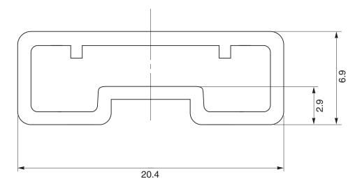
MM450-01A Length: 495±2.0 Thickness: 1.0<sup>+0.3</sup><sub>-0.2</sub> Tolerance: ±0.4
