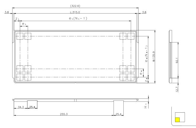
The pin1 is located in the hatching portion
