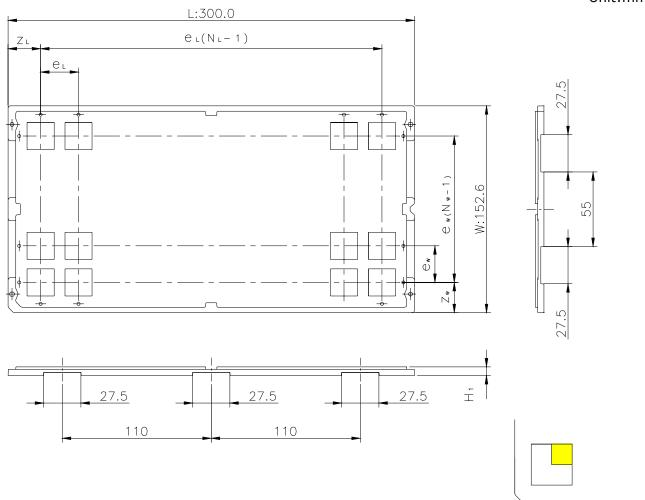
The pin1 is located in the hatching portion
