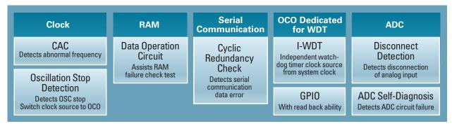
CAC: Clock frequency accuracy measurement circuit OCO: On-chip oscillator
