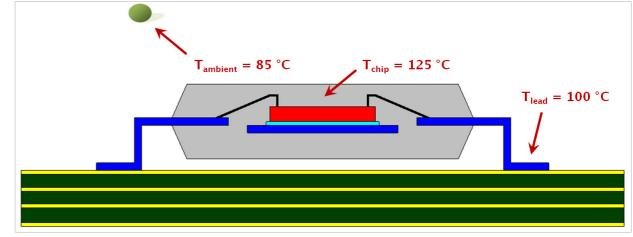
Figure 1: Package on a PCB with relevant temperature-monitor points 0.040" is 20,500.  $i = kD^{\overline{2}}$
