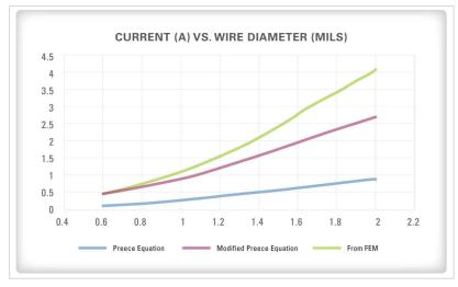
where  $\rho$  is the wire's resistivity (2.44x10-8  $\Omega$ -m for gold and 1.68x10-8  $\Omega$ -m for copper), D is the wire diameter, l is the wire length, and  $\Delta T$  is the temperature difference between the wire's two ends, which we assume to be a constant for a maximum current-capacity calculation. Simplifying even further,
