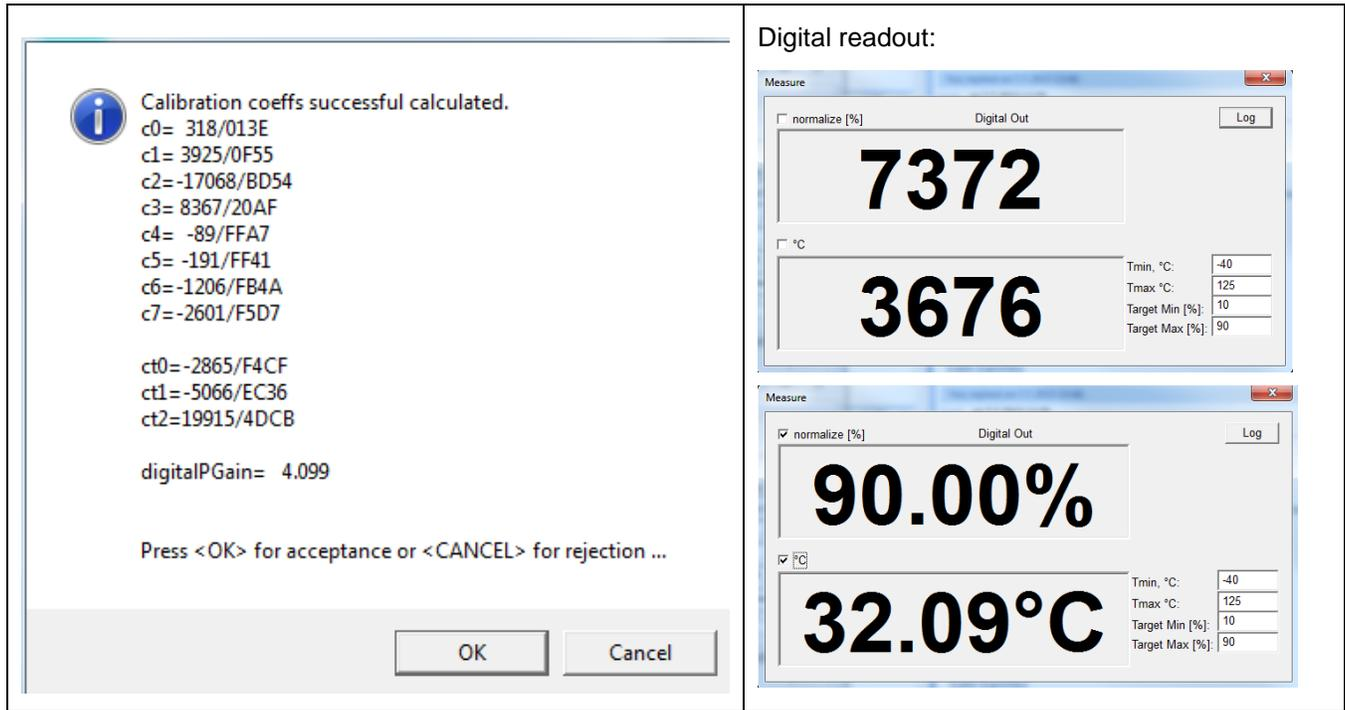
After successful calibration, the output of the SSC IC should vary between the target limits specified during calibration. For digital data, the readout values match the resolution of the data format used.
