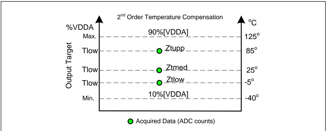
The upper and lower limits (Max. and Min.) are usually selected as 10% and 90% of the ADC reference voltage (the analog voltage supply). Note that this varies depending on the SSC IC. In this input range, the ADC has the best performance for linearity.
