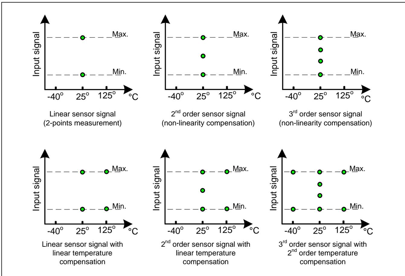
The calibration point configuration can be any setup from 2-points linear calibration to 3<sup>rd</sup> order non-linearity compensation and 2<sup>nd</sup> order temperature dependency compensation.
