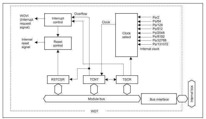
Figure 2 Block Diagram of Watchdog Timer
