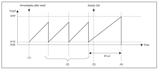
Figure 3 Watchdog Operation by Watchdog Timer Function
