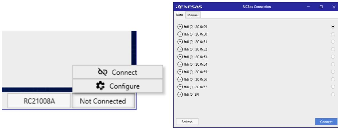
If the EEPROM is detected, then you are ready to program. Refer to the EEPROM user’s manual about which jumpers to set to add the EEPROM to the I<sup>2</sup>C bus.
