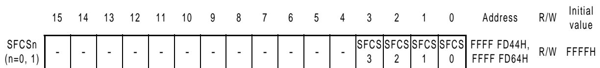
Figure 2-9: Chip Select Data Buffer Registers (SFCS0, SFCS1) Format
