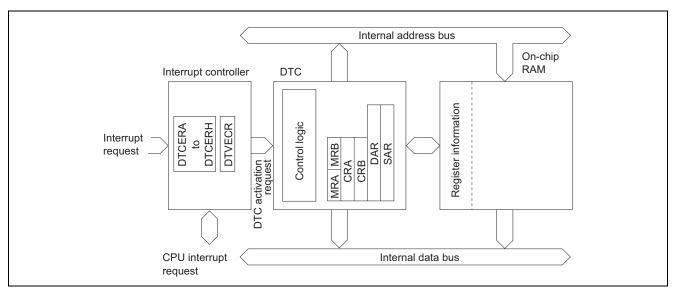
Figure 5 Block Diagram of DTC
