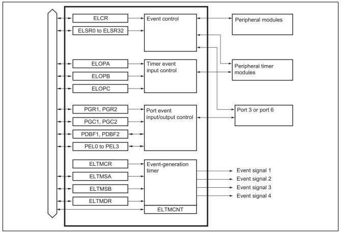
Figure 3 Block Diagram of Event Link Controller
