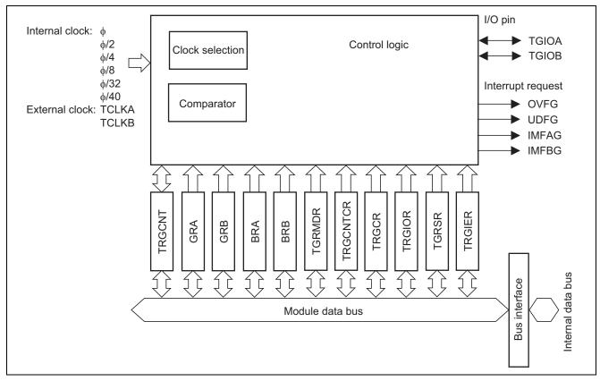
Figure 4 Block Diagram of Timer RG
