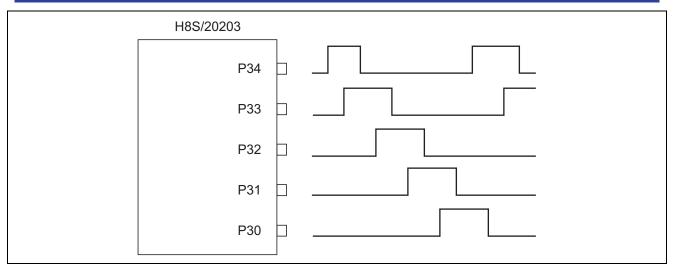
Figure 2 Port Group Output in Timing Pattern Controller Operation
