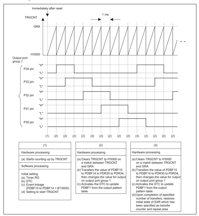
Figure 9 Principle of Operation in the Sample Task
