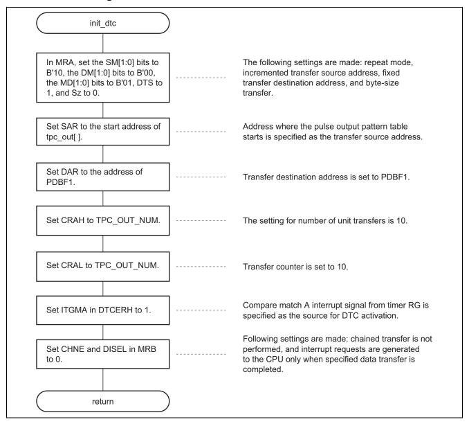
Using Timer RG and Port Output for Timing Pattern Controller Operation
