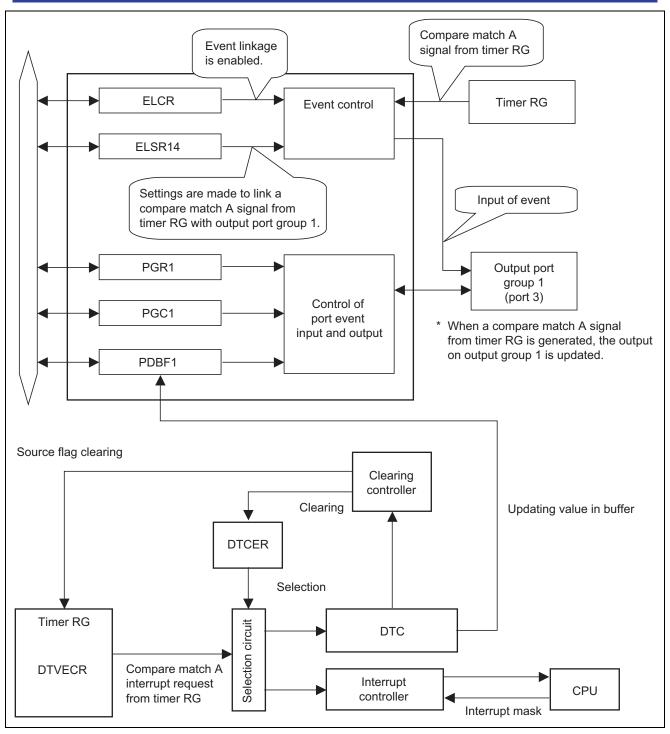
Figure 1 Schematic View of How Timer RG and Port Group Output are Used to Set up TPC Operation
