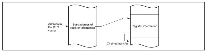
Figure 8 Correspondence between the Address in a DTC Vector and Register Information
