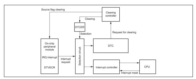
Figure 6 Block Diagram of DTC Activation Source Control
