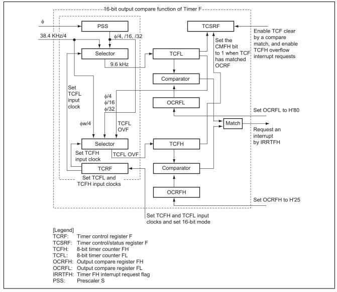
Figure 2 Block Diagram of Timer F Compare Match Function
