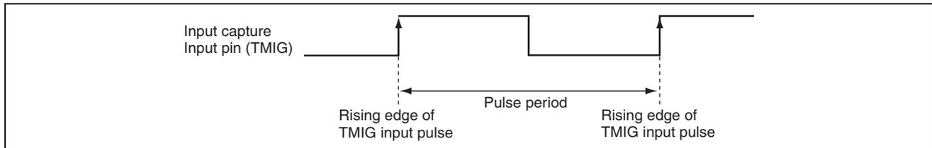
Figure 1.1 Measurement of Input Pulse Period
