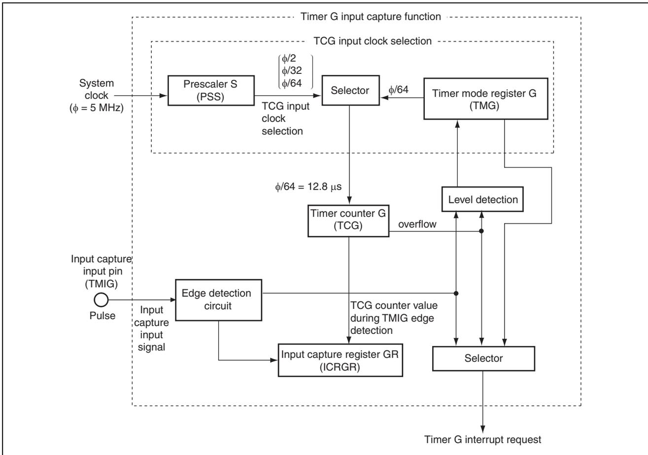
**Figure 2.1 Block Diagram of Timer G Input Capture Function**
