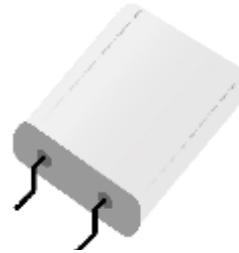
Figure 4- The HC/49U or UM1 crystal can be ordered with gull-wing leads for surface mounting.
