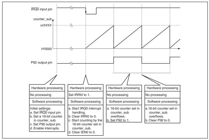
Figure 3.1 Operation Principle of Starting Counter Incrementation by External Interrupt
