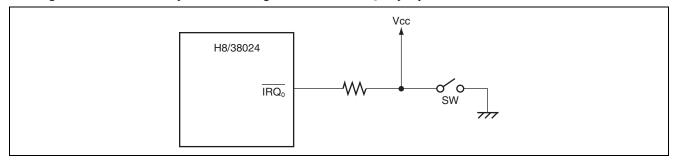
Figure 1.1 Example of Connecting a Switch to IRQ0 Input Pin
