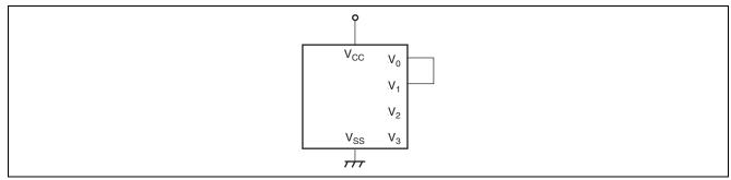
Figure 3.1 LCD Power Supply Pin Connection When the On-Chip Power Supply Circuit is Used
