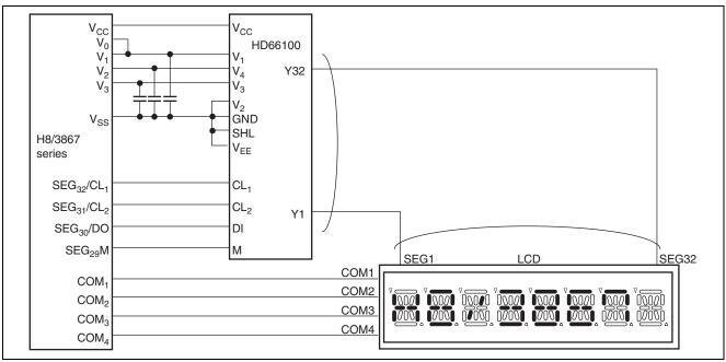
Figure 1.1 Examples of HD66100 and LCD Module Connection by Segment Extension, and LCD Display
