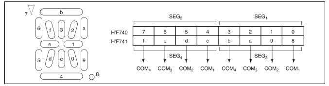
Figure 2.5 Relationship between LCD Light On/Off and Corresponding LCD RAM Setting Values
