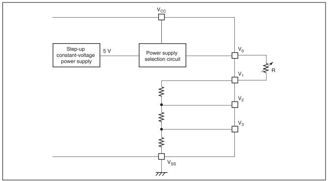
Figure 3.2 Block Diagram of LCD Drive Power Supply Unit
