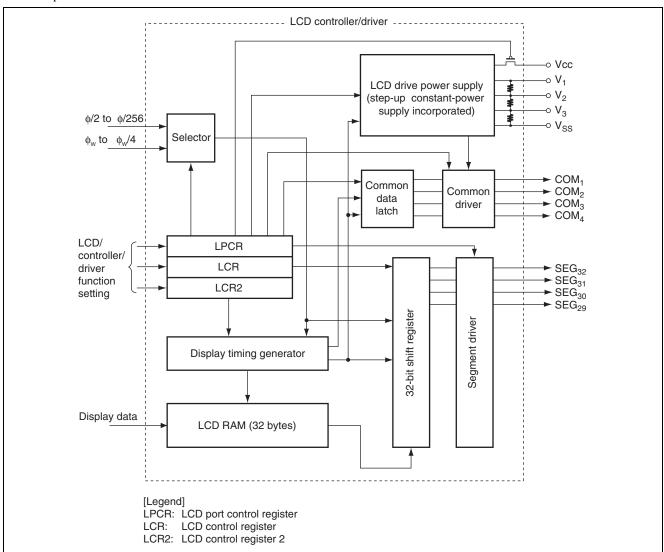
Figure 2.1 Block Diagram of LCD Controller/Driver in Segment External Extension
