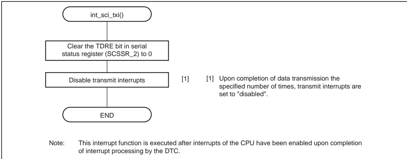
**Figure 14 Flow for Handling Transmit Interrupts in Clock Synchronous Mode**
