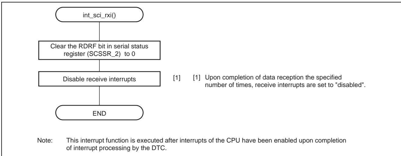
**Figure 15 Flow for Handling Receive Interrupts in Clock Synchronous Mode**
