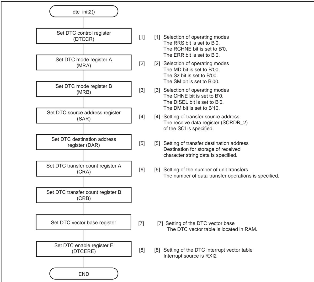
**Figure 11 Flow 2 of DTC Initialization (before Receive Operation)**
