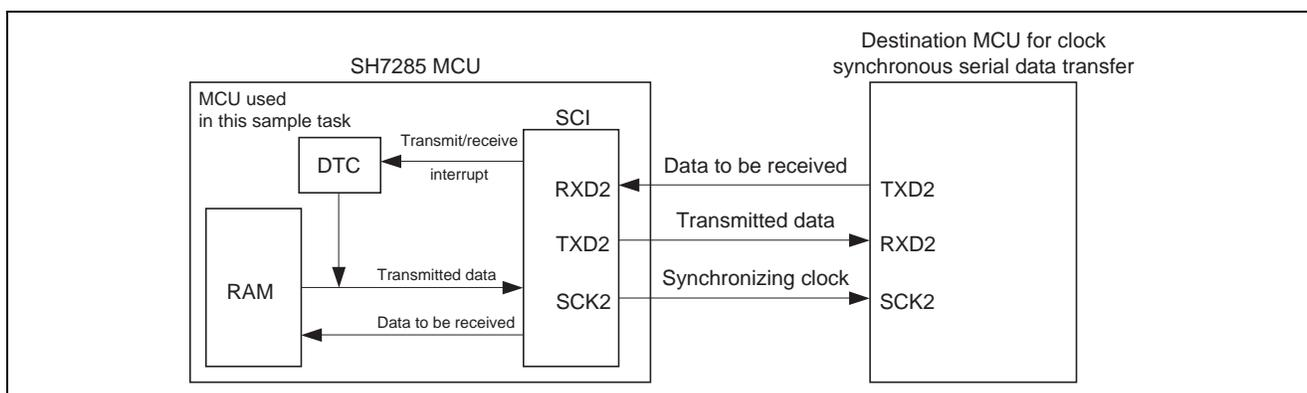
**Figure 1 Example of Connection for Using the DTC in Transmission and Reception of Serial Data in Clock Synchronous Mode**
