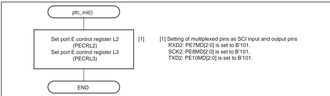
**Figure 13 Flow for Setting Up the Pin Function Controller**
