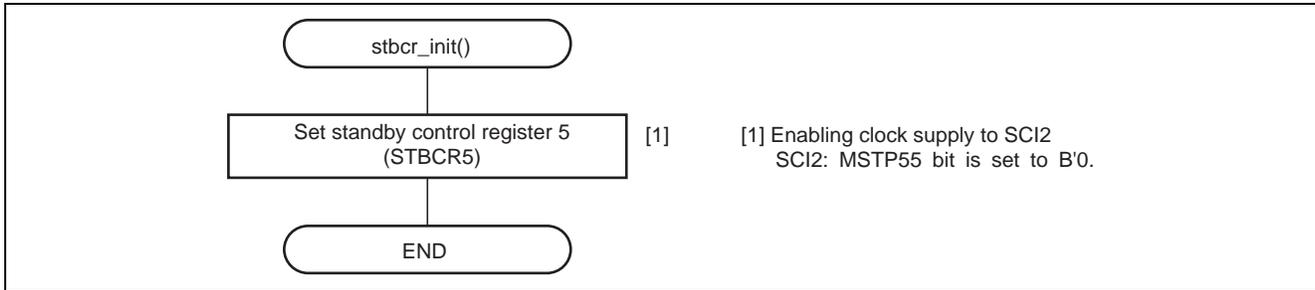
**Figure 9 Flow of Setting for Release from Module-Standby Mode**
