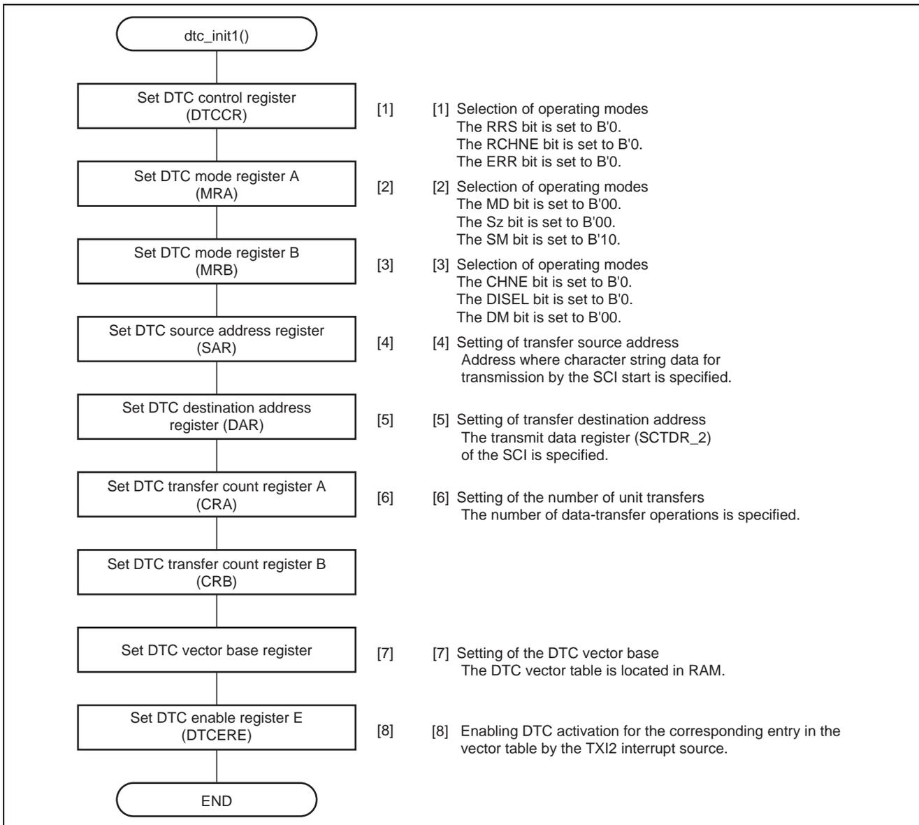
**Figure 10 Flow 1 of DTC Initialization (before Transmission)**
