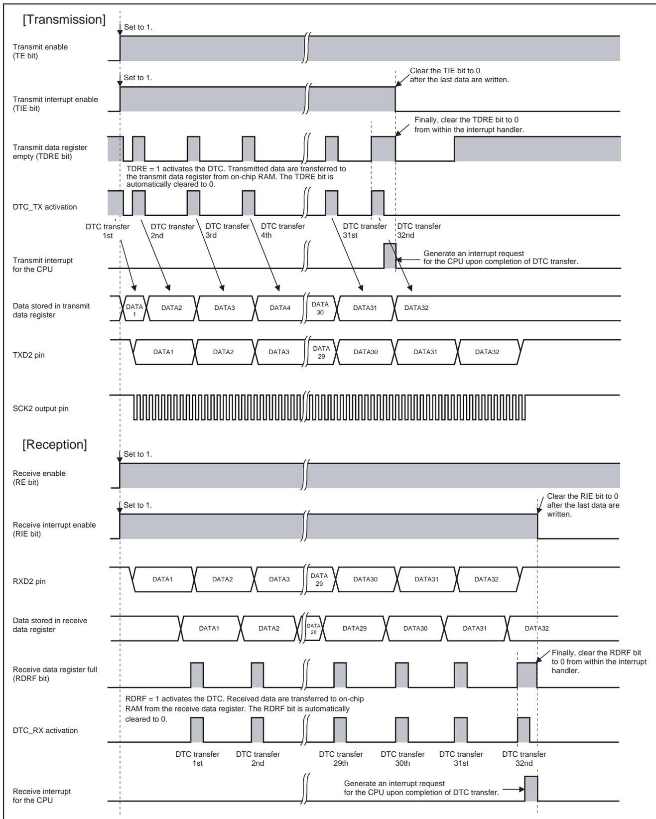
**Figure 7 Principles of Operation**
