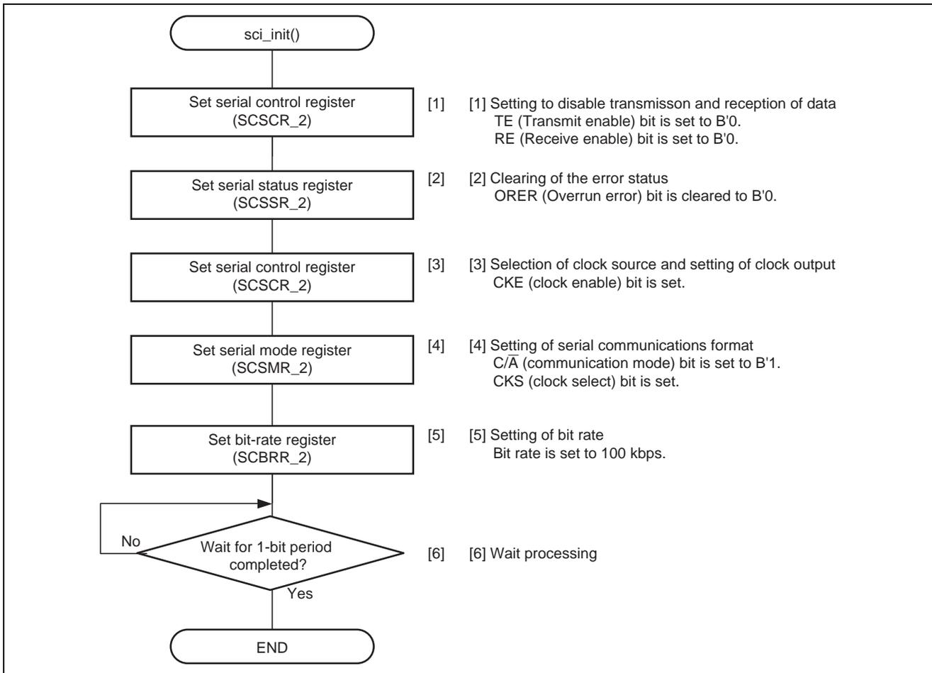
**Figure 12 Flow for Initialization of Data Transmission and Reception in Clock Synchronous Mode**
