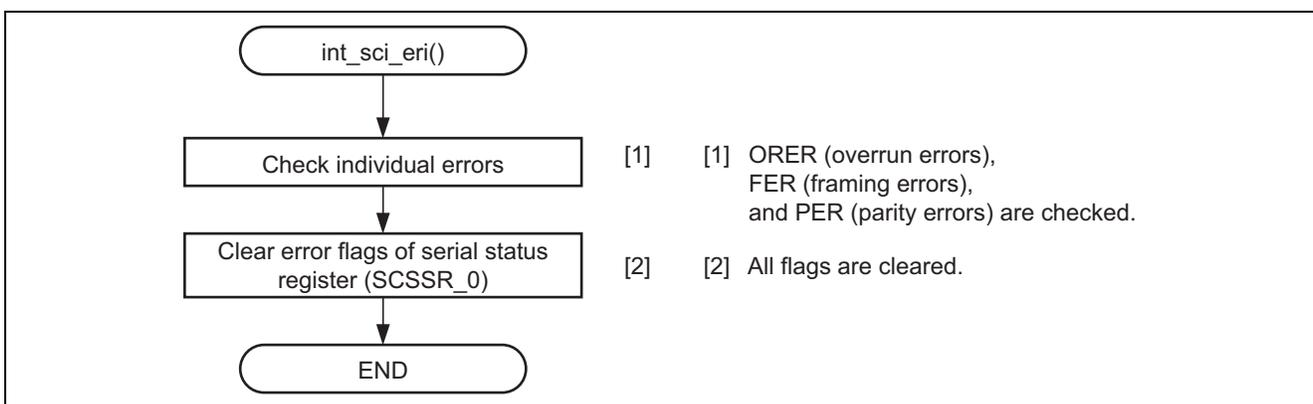
**Figure 16 Flow for Handling Receive Error Interrupts**
