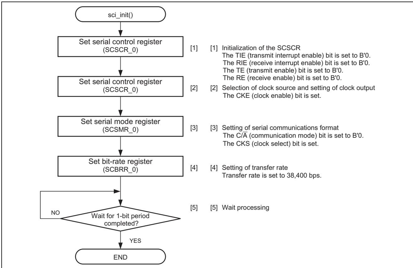
**Figure 13 Flow for Initialization of Data Transmission and Reception in Asynchronous Mode**
