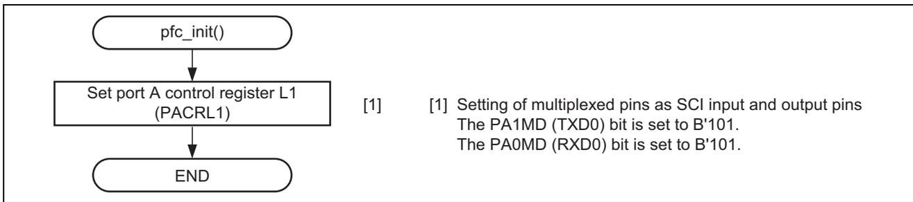
**Figure 10 Flow for Setting up the Pin Function Controller**
