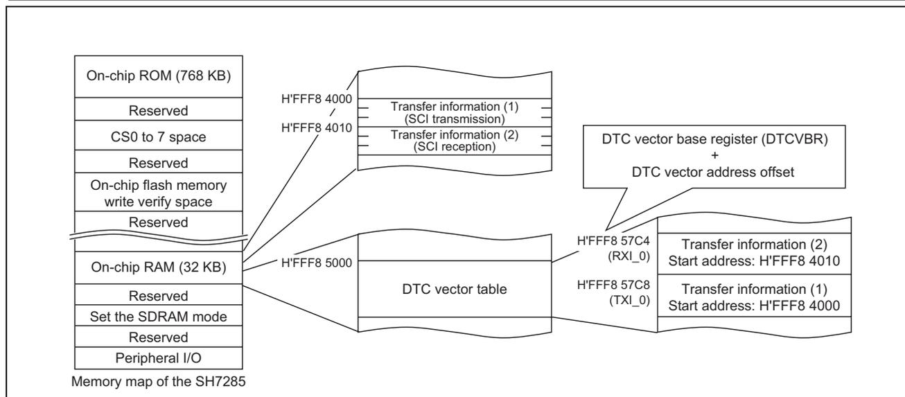
**Figure 6 Image of Arrangement of Transfer Information in Memory**
