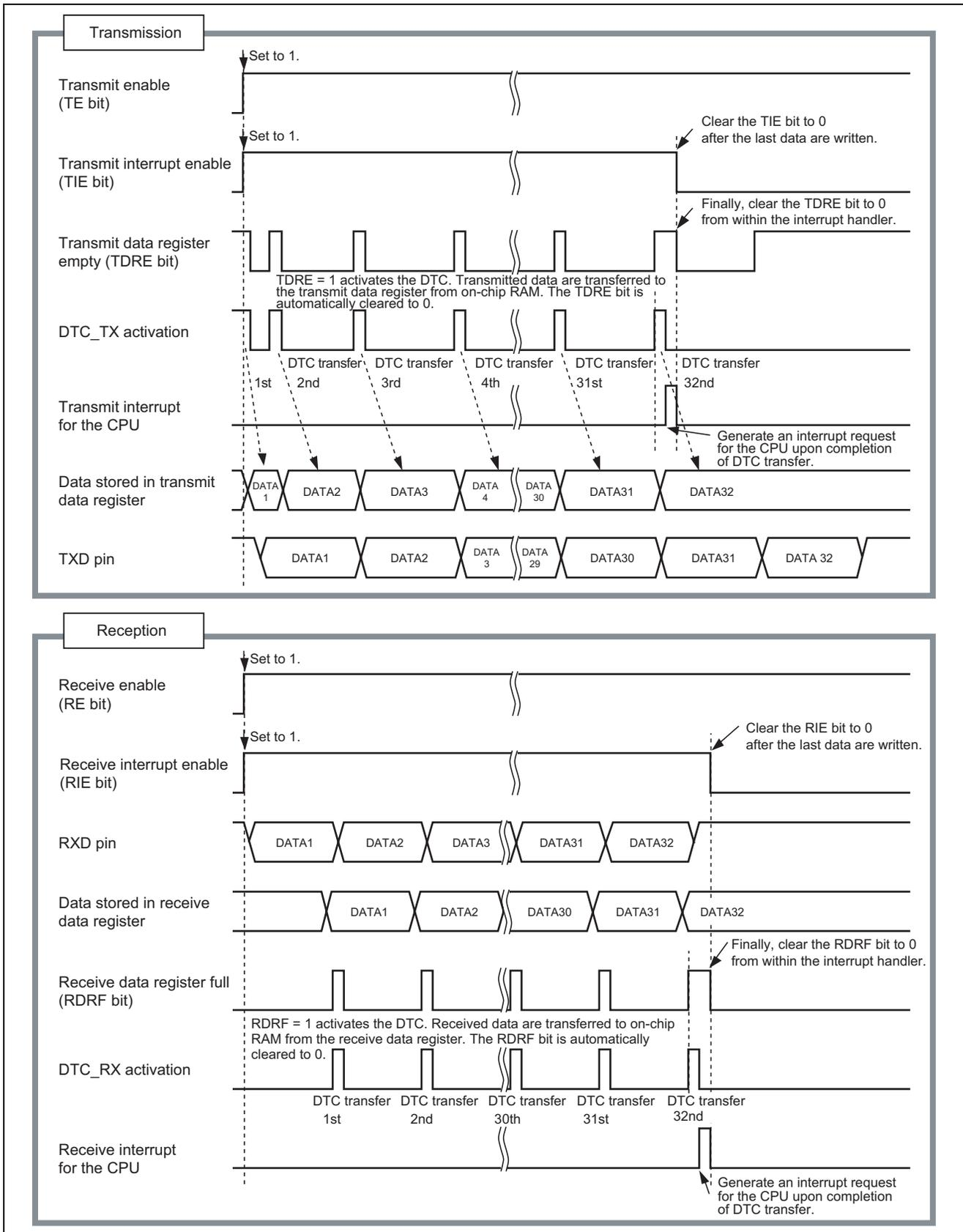
Figure 7 Principles of Operation
