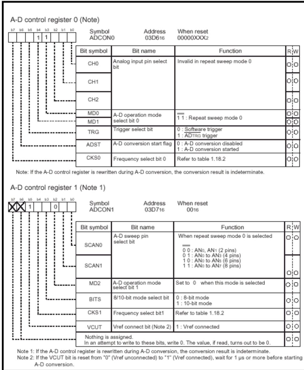
Figure 2 ADC control registers in Repeat Sweep Mode 0
