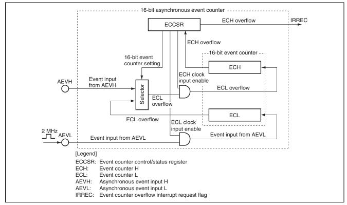
Figure 2.1 Block Diagram of Asynchronous Event Counter
