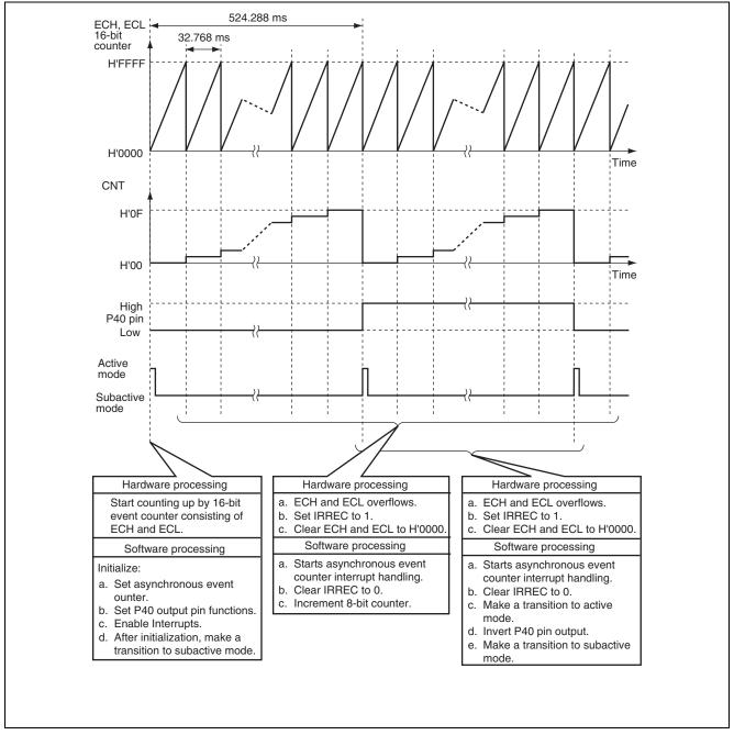
Figure 3.1 Operation Principle of Asynchronous Event Counter
