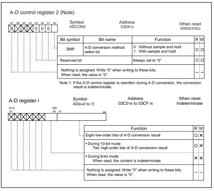
Figure 3 A-D Converter Related Register
