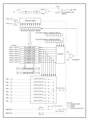
Figure 1 Internal Circuitry for ADC Block—Overview
