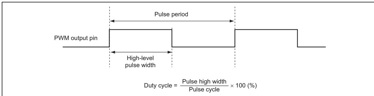
**Figure 1 Duty Cycle Pulse Output By 14-Bit PWM Function**
