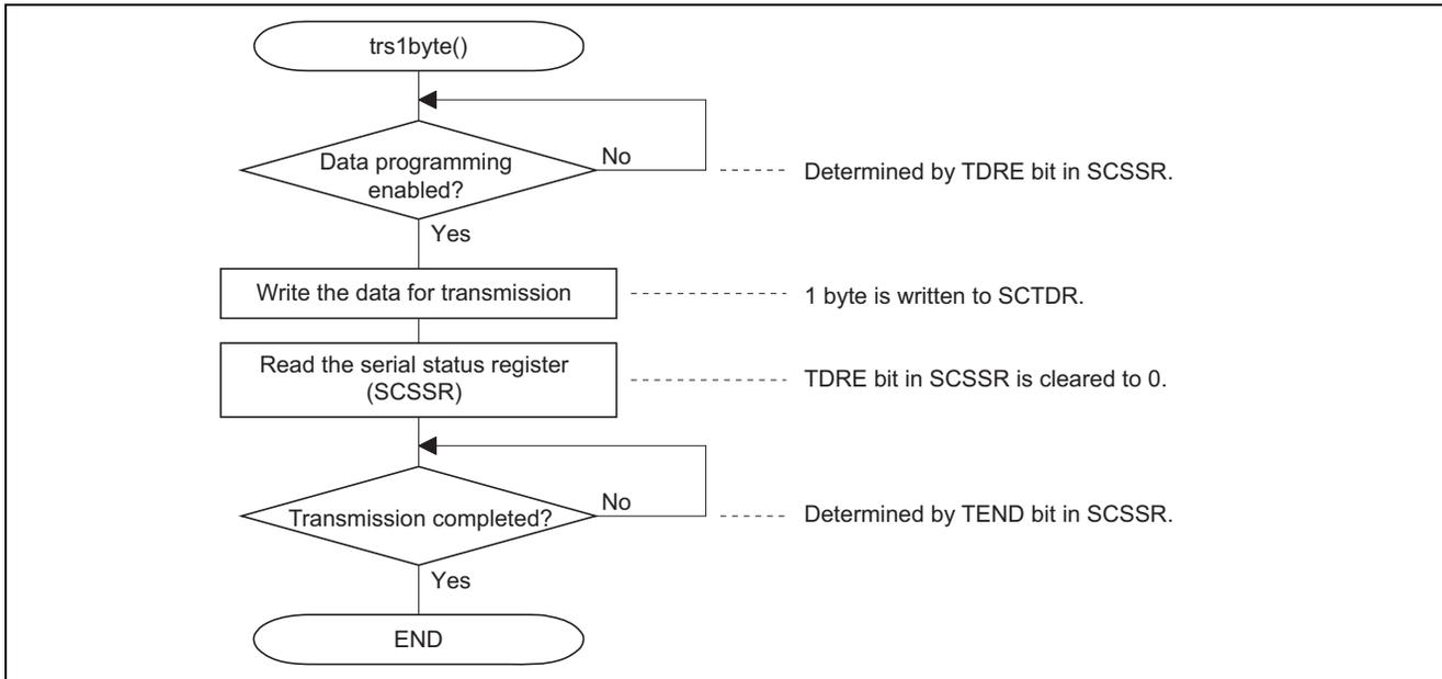
Figure 10 Processing by the SCI\_1 1-Byte Transmission Routine
