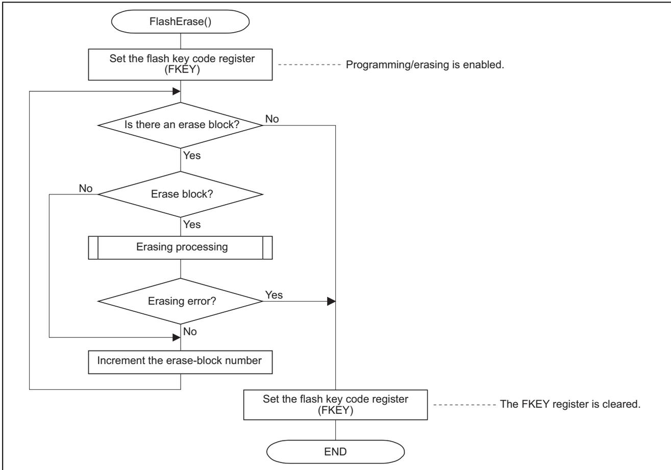
Figure 15 Processing by the Flash Erasing Routine
