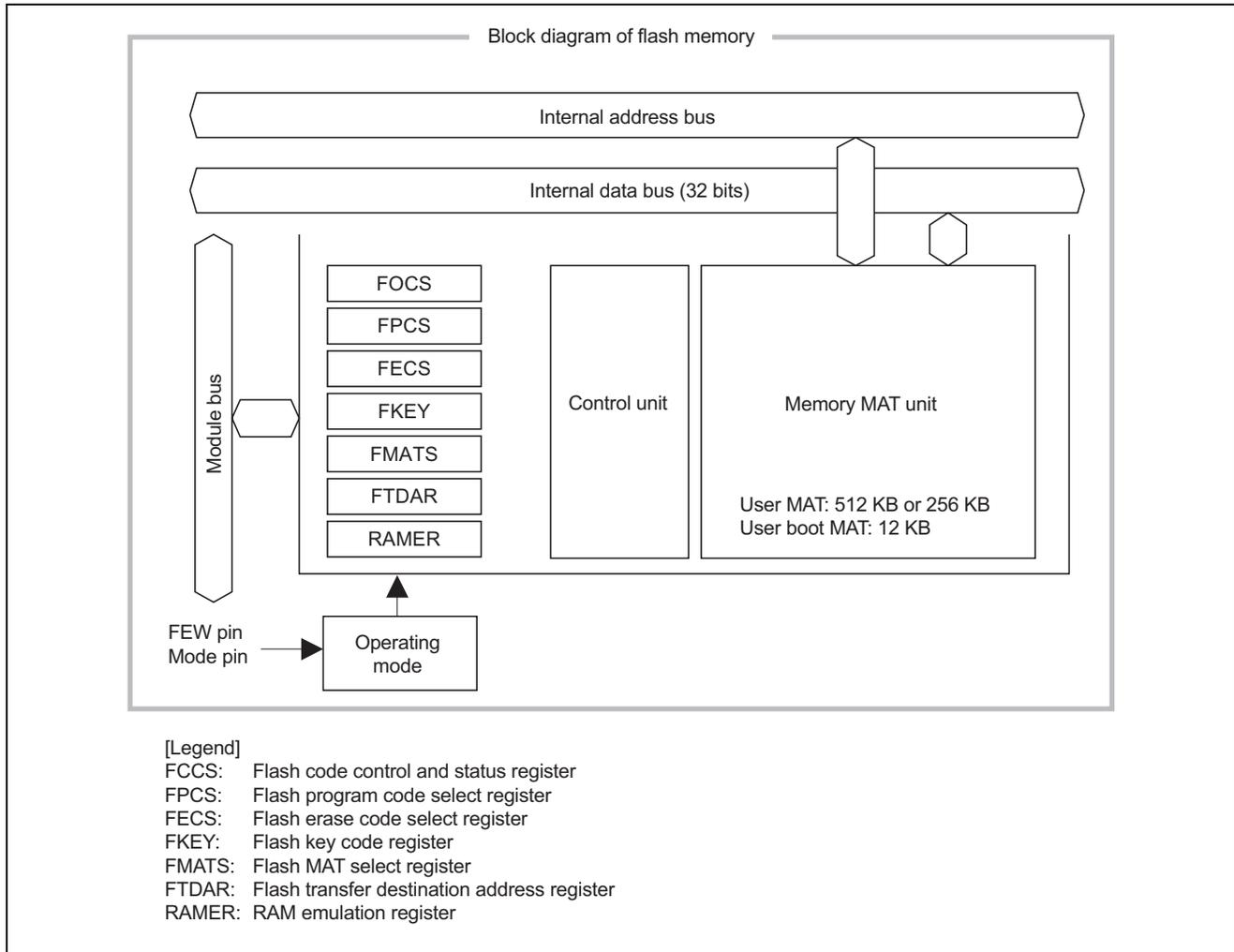
Figure 2 Block Diagram of Flash Memory
