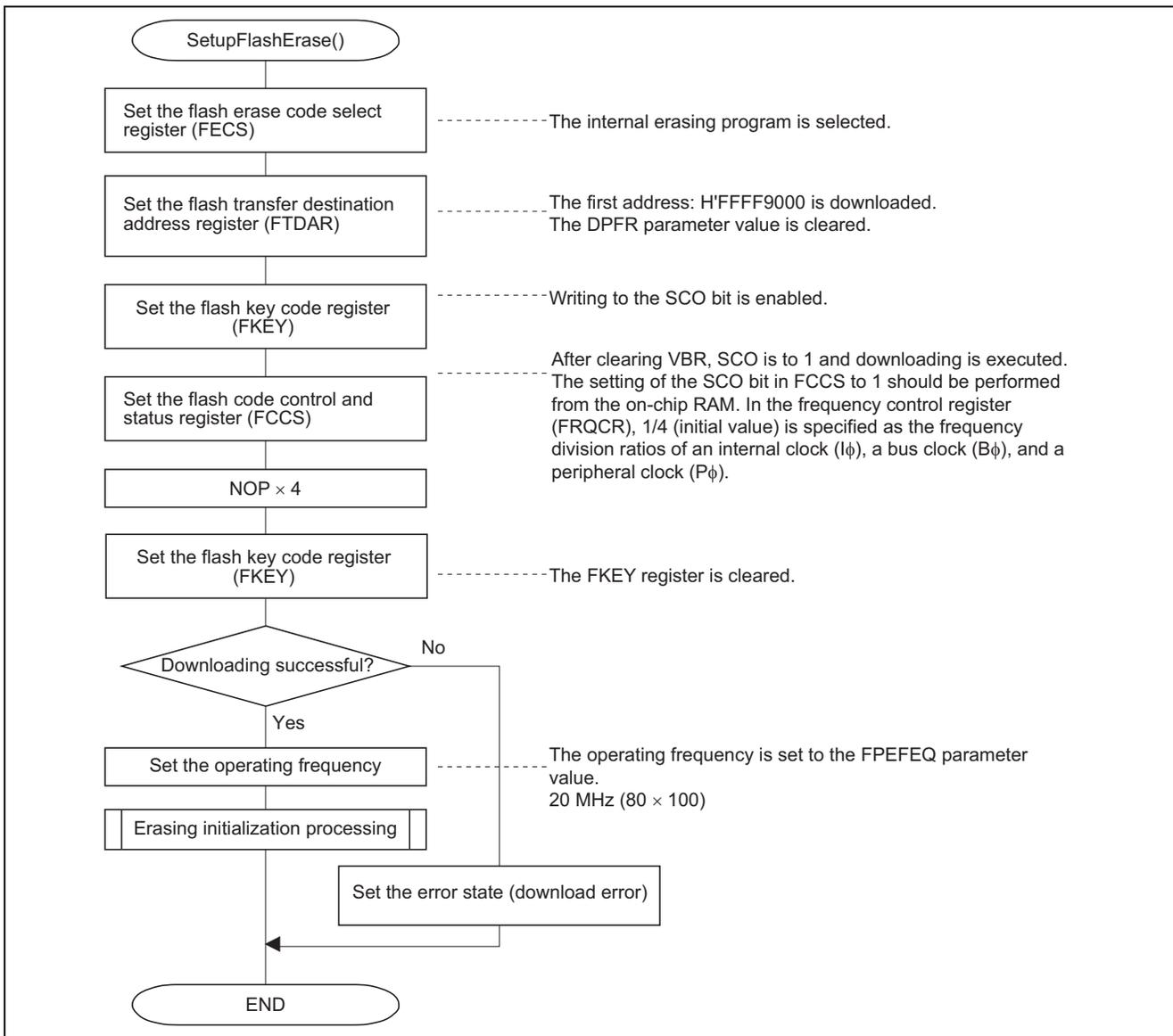
Figure 14 Processing by the Erasing Program Downloading and Initialization Routine
