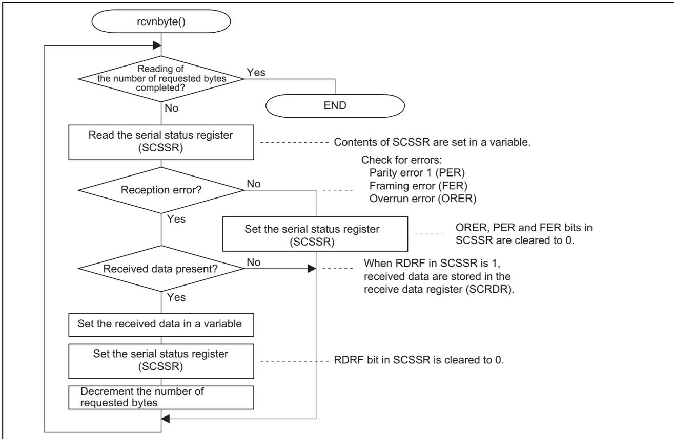
Figure 9 Processing by the SCI\_1 n-Byte Reception Routine
