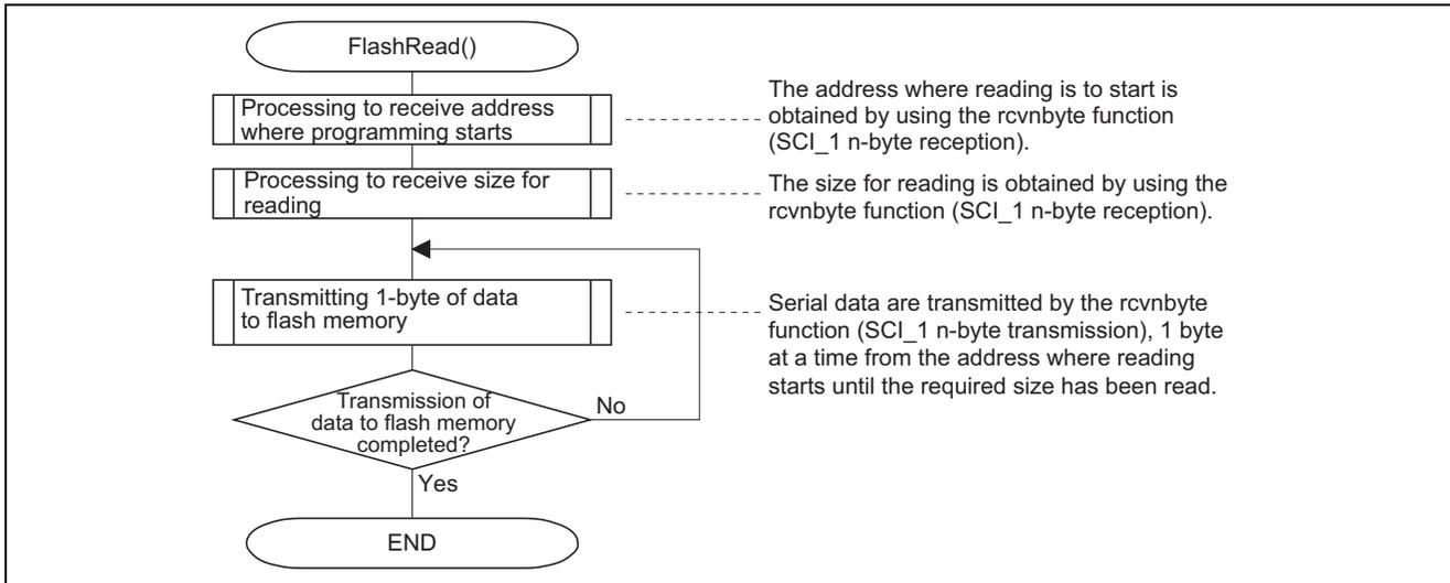
Figure 13 Processing to Read Flash Memory
