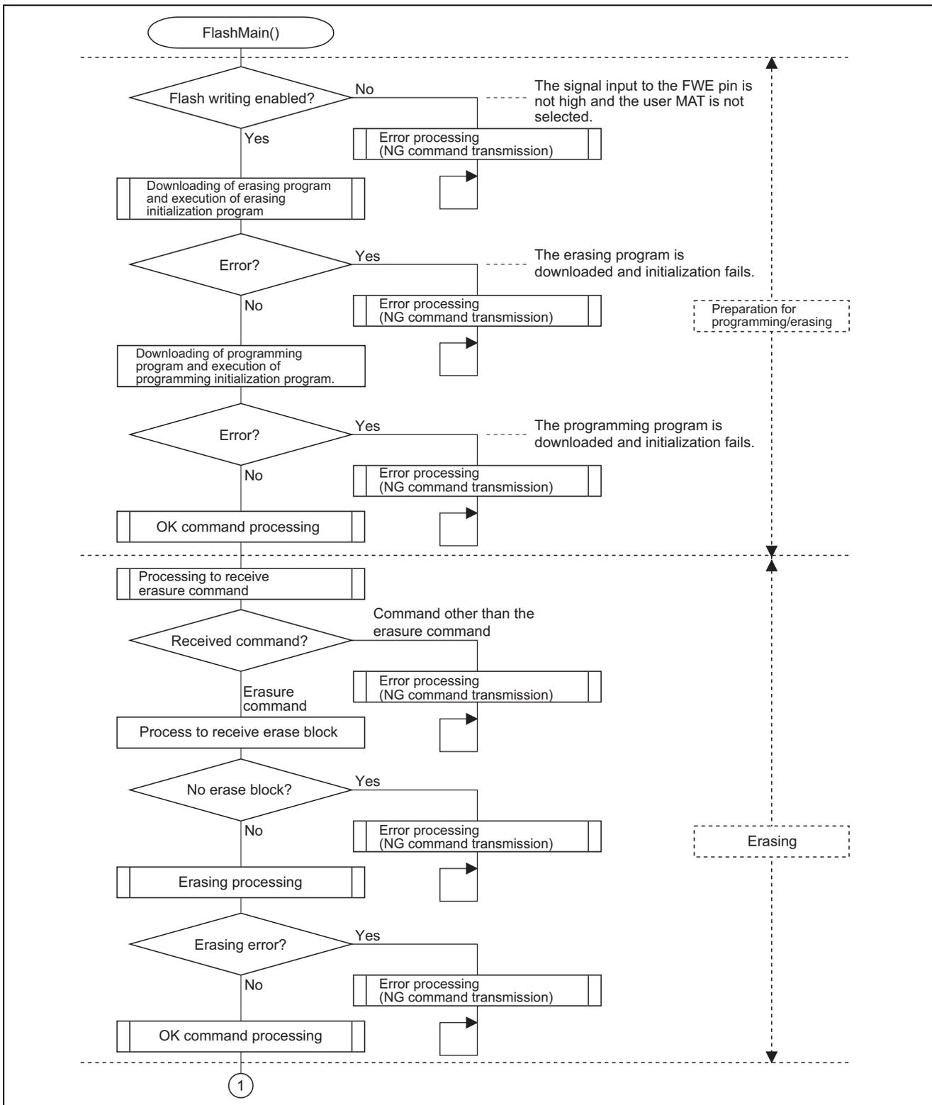
Figure 11 Processing by the Main Routine for Flash Programming (1)
