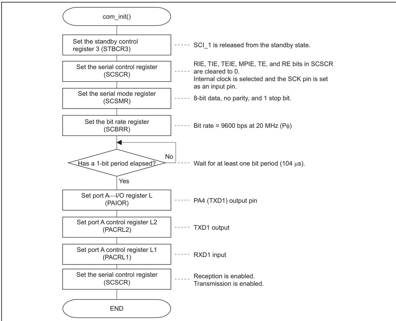
Figure 7 Processing by the SCI Channel 1 Initialization Routine
