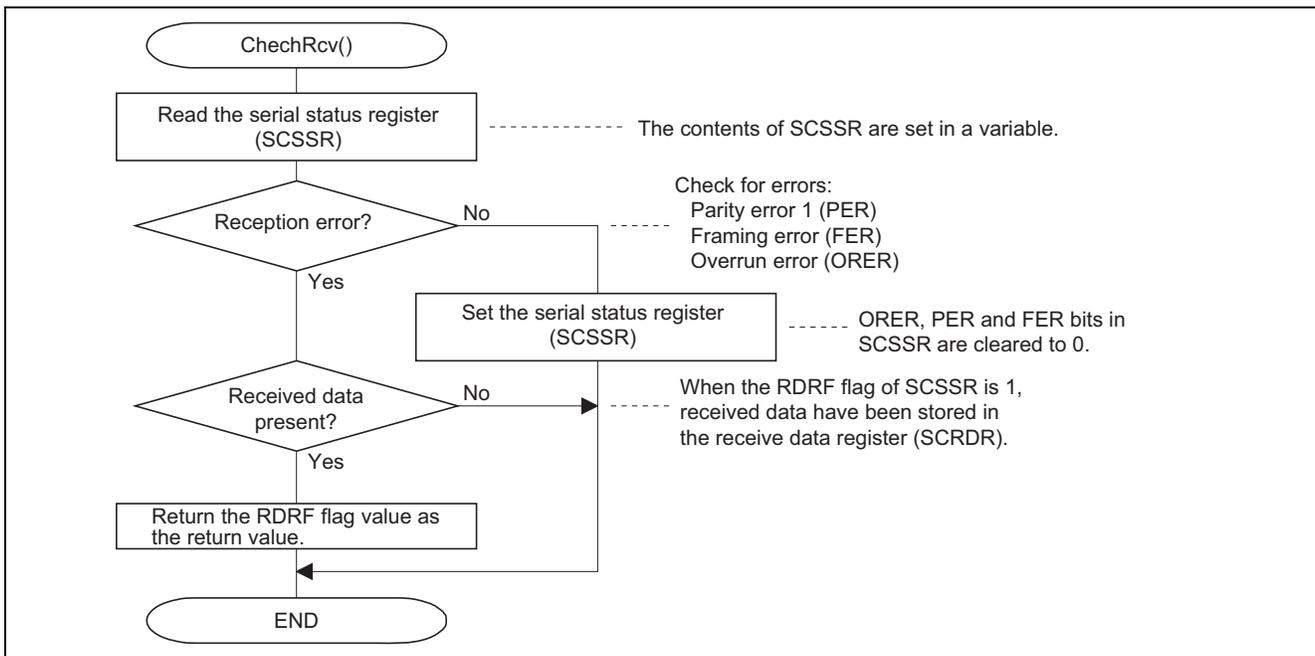
Figure 8 Processing by the Routine to Check for SCI\_1 Received Data
