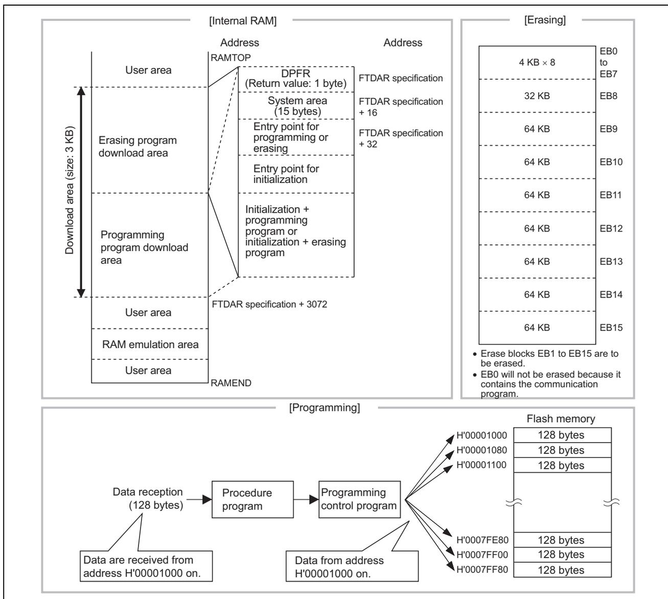
Figure 3 Flash Erasing/Programming Specifications
