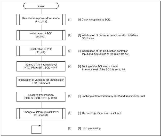
Figure 4 Flow of Processing by the Sample Task
