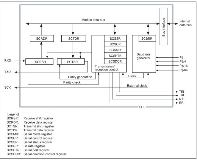
Figure 2 Block Diagram of the SCI
