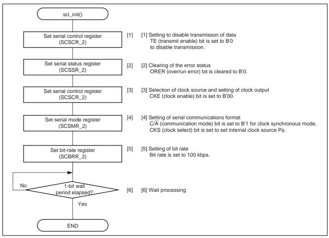
Figure 6 Flow for Initialization of Data Transmission in Clock Synchronous Mode
