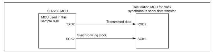
Figure 1 Connection Example for Transmission by the SCI in Clock Synchronous Mode
