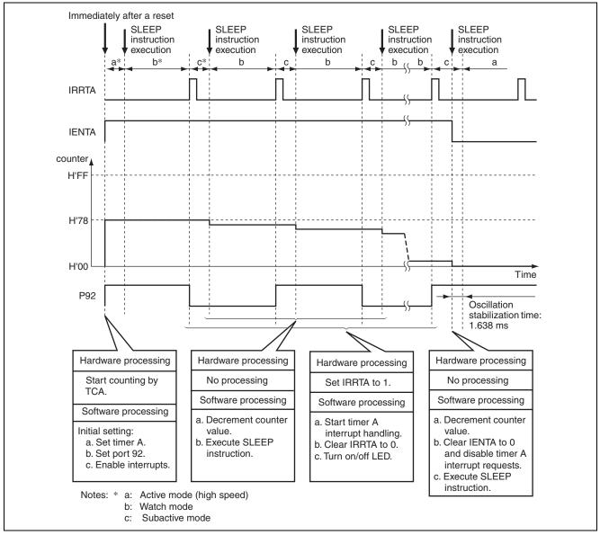
Figure 3.1 Principle of Operation of Making Transition to Watch Mode
