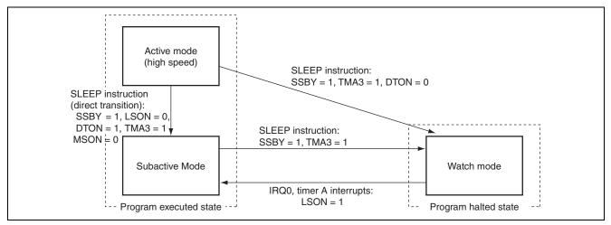
Figure 2.1 Mode Transition from/to Watch Mode
