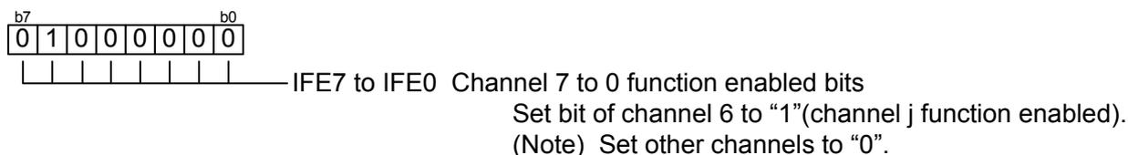
(8) ICOC0IC register (interrupt disable setting /interrupt request bit clear)
