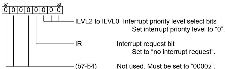
(9) G1IE0 register (interrupt enabled register reset)
