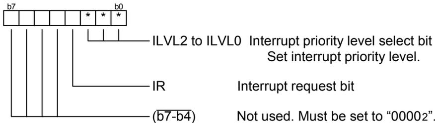
(\*) Use "OR" instruction so that the interrupt request bit is not changed when setting the interrupt priority level.
