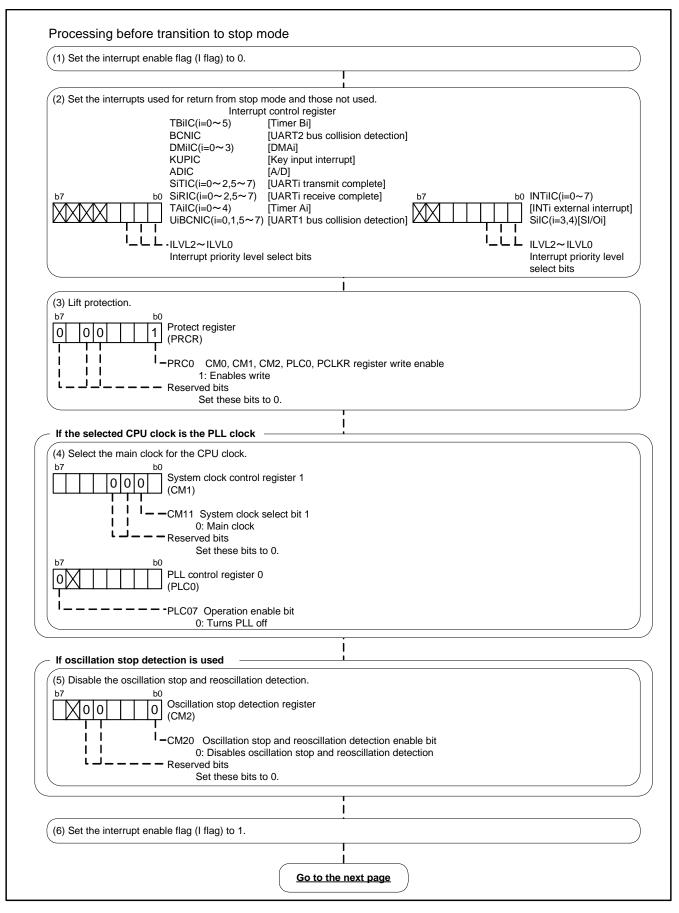
Figure 1.1 Example for Setting Up Registers to Enter Stop Mode
