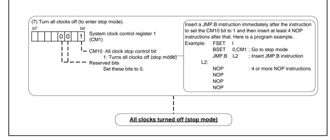
Figure 1.2 Example of Register Setup for Entering Stop Mode
