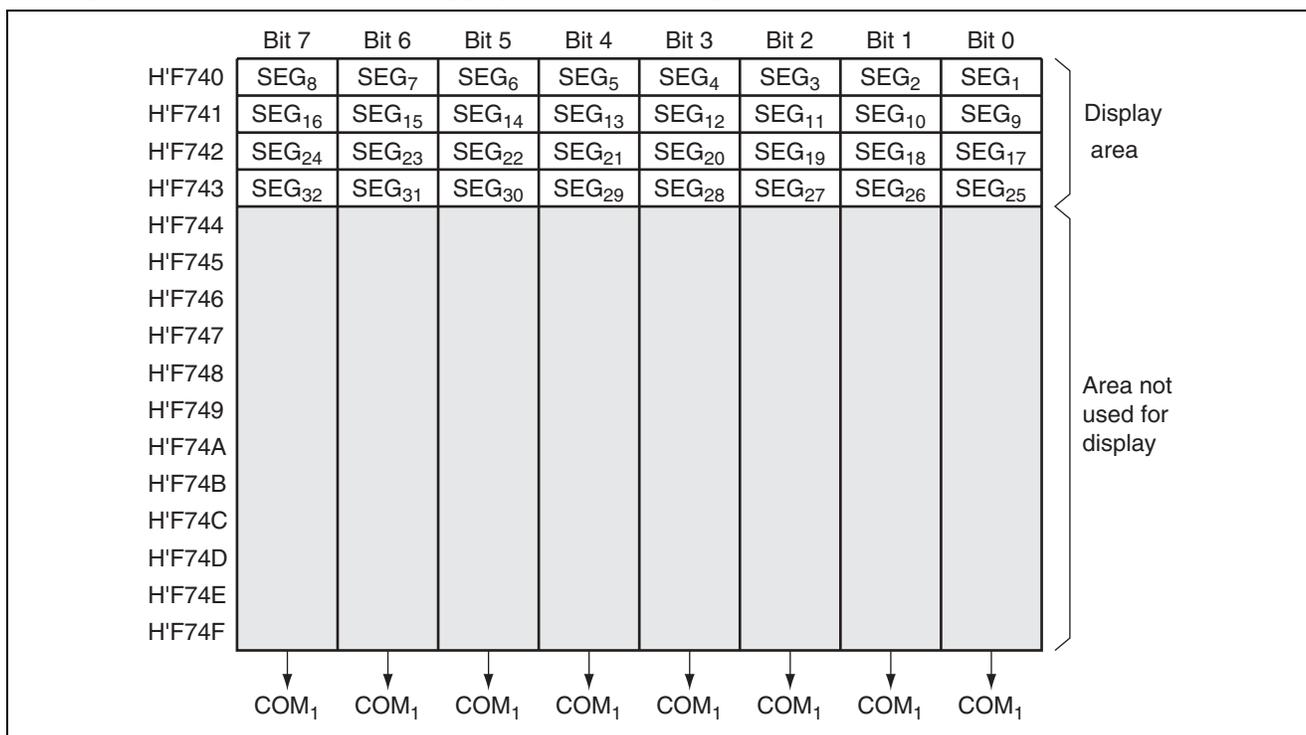
**Figure 2.3 LCD RAM Mapping under Static Driving**
