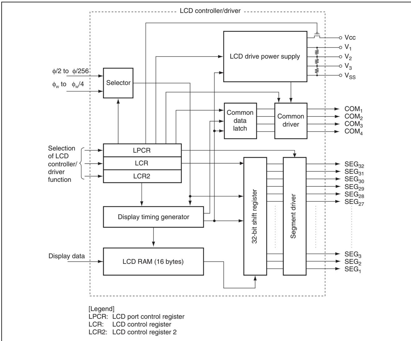
Figure 2.1 Block Diagram of LCD Controller/Driver
