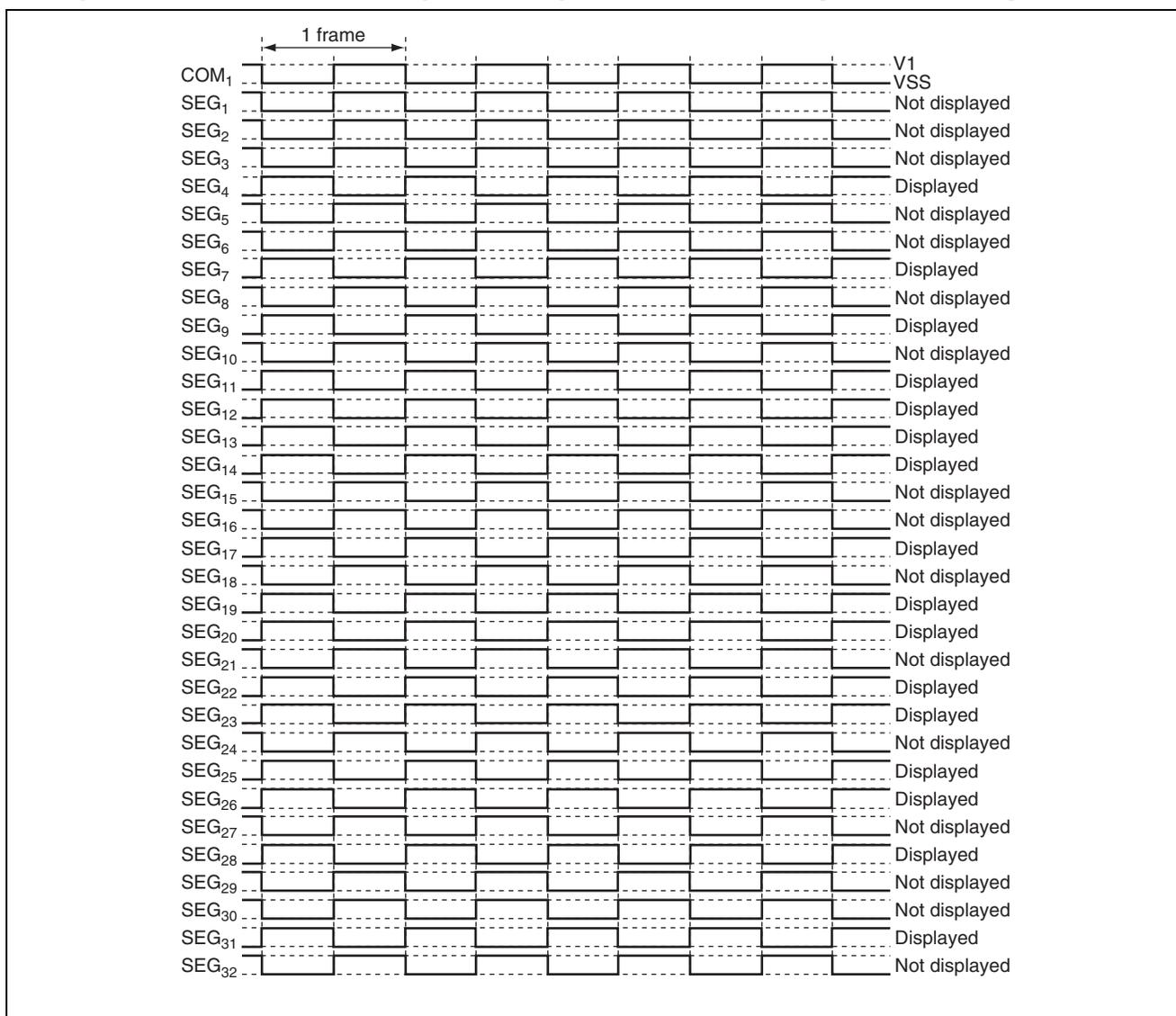
Figure 3.1 Waveforms of Segment Drive Signals
