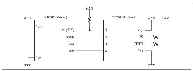
Figure 1 Example of Connection between the SH7085 and EEPROM
