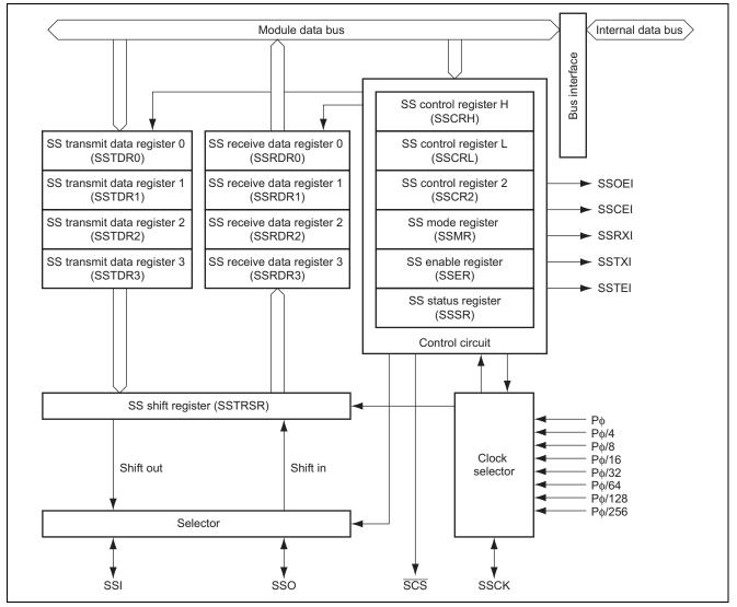
Figure 2 Block Diagram of the SSU Module
