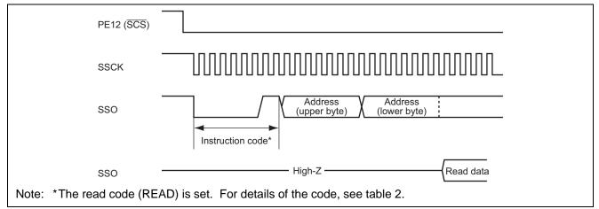
Figure 3 Communication Processing for Reading Data from the EEPROM
