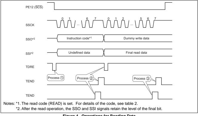
Figure 4 Operations for Reading Data
