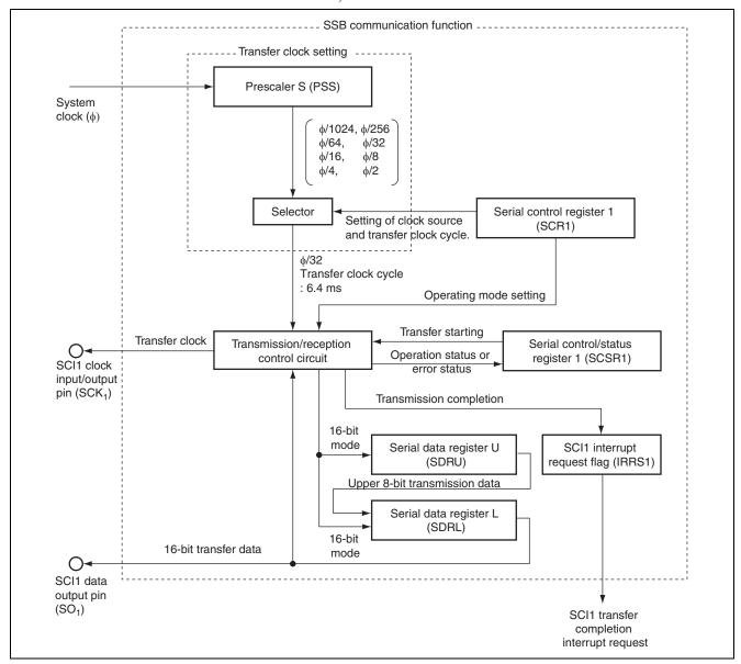
Figure 2.1 Block Diagram of SSB Communication Function
