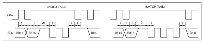
Figure 2.3 Hold and Latch Tail Output Waveforms
