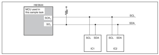
Figure 1.1 Example of SSB Connection
