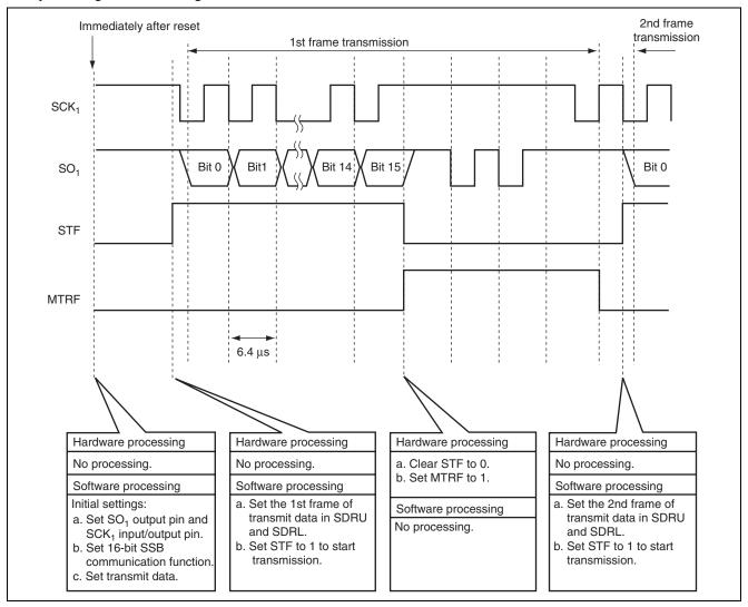
Figure 3.1 Principle of Operation of SSB Communication
