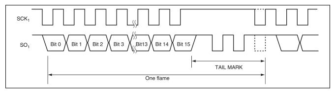
Figure 2.2 Transfer Format (When SNC1 = 0, SNC0 = 1 and MRKON = 1)
