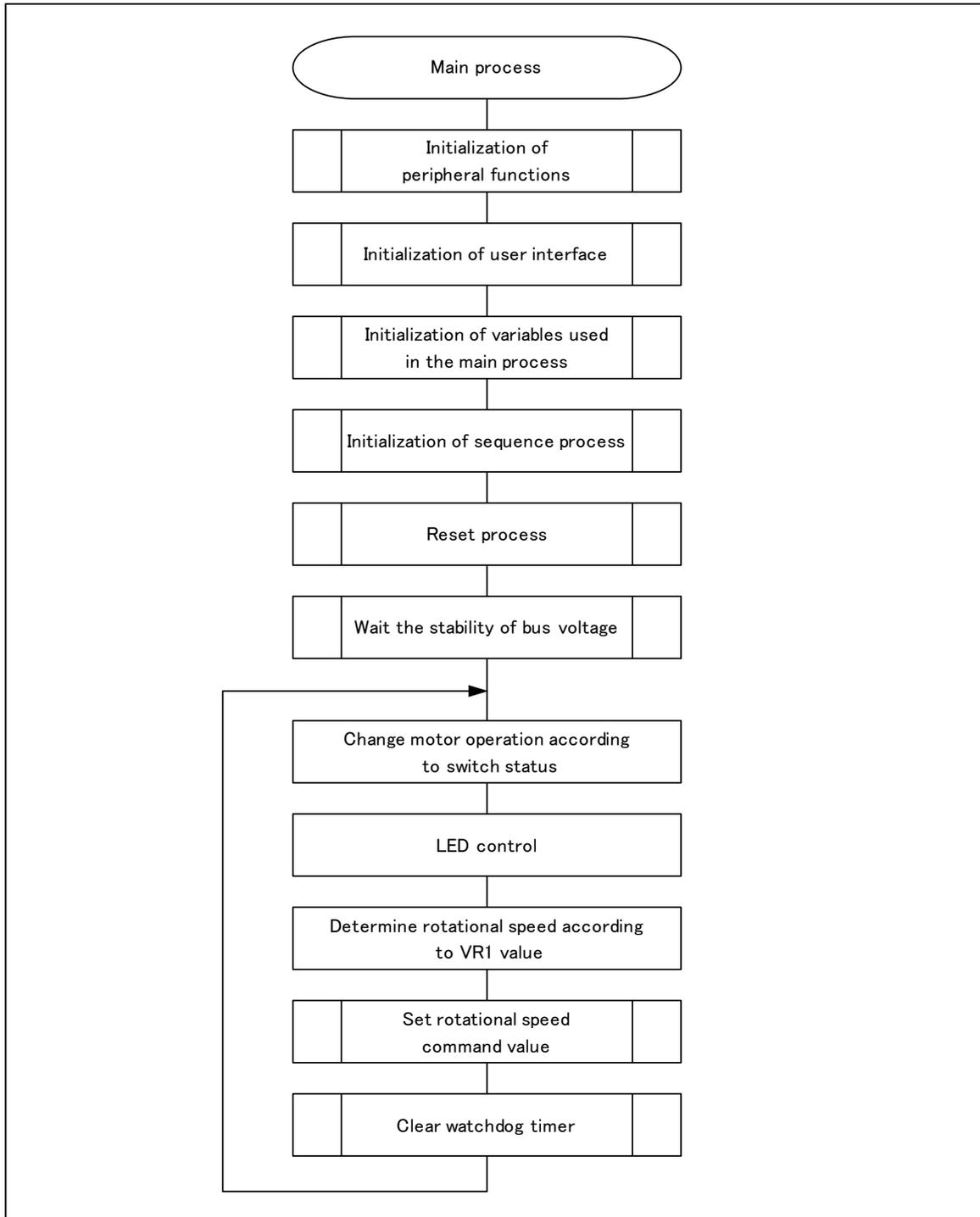
Figure 3-7 Main Process Flowchart
