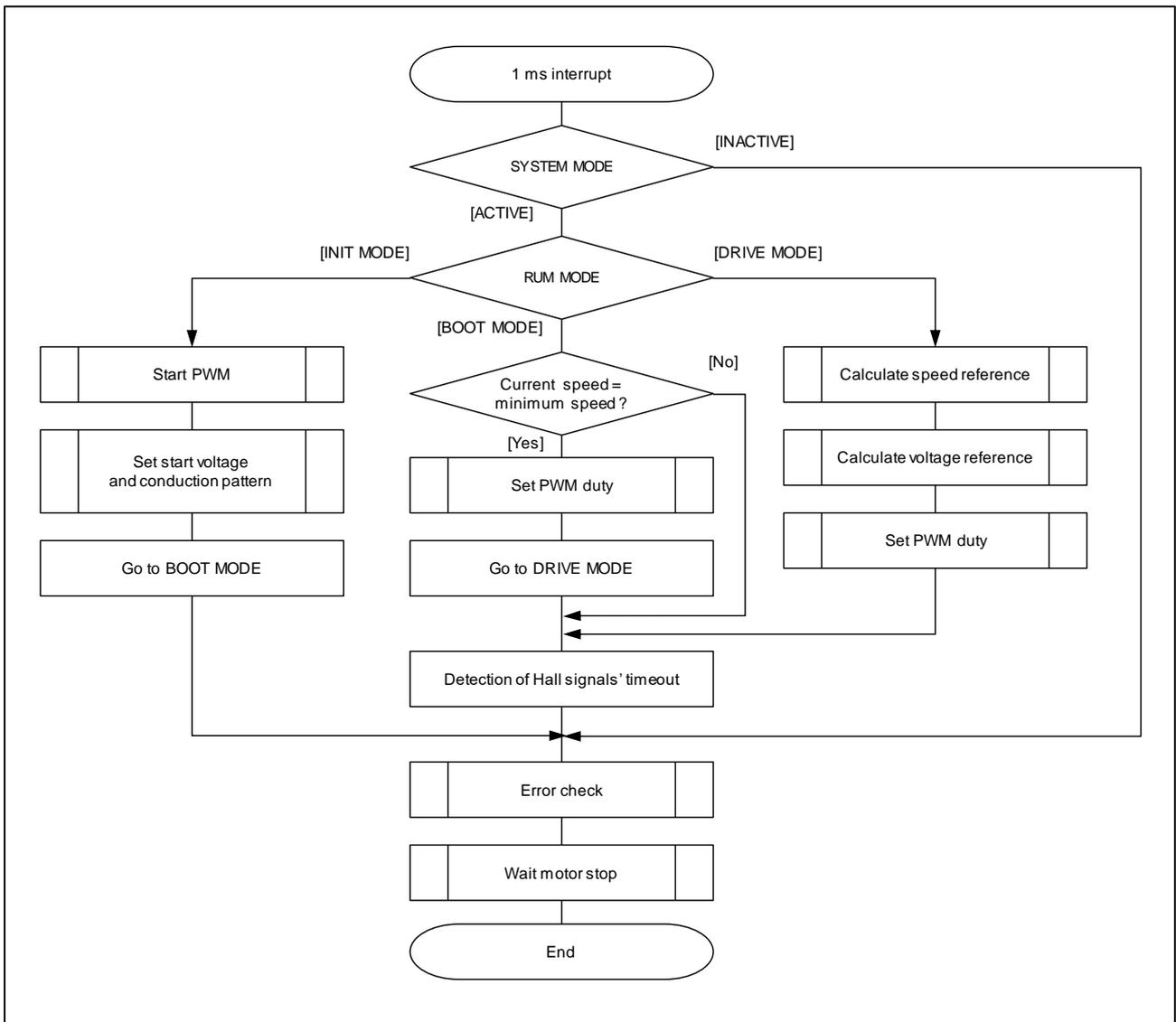
Figure 3-9 1 [ms] Interrupt Handling
