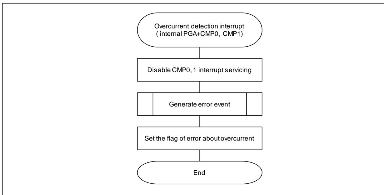
Figure 3-11 Over Current Detection Interrupt Handling (PGA+CMP0, CMP1)
