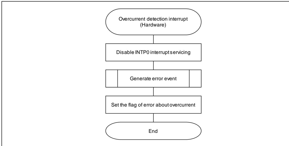
Figure 3-10 Over Current Detection Interrupt Handling (INTPO)
