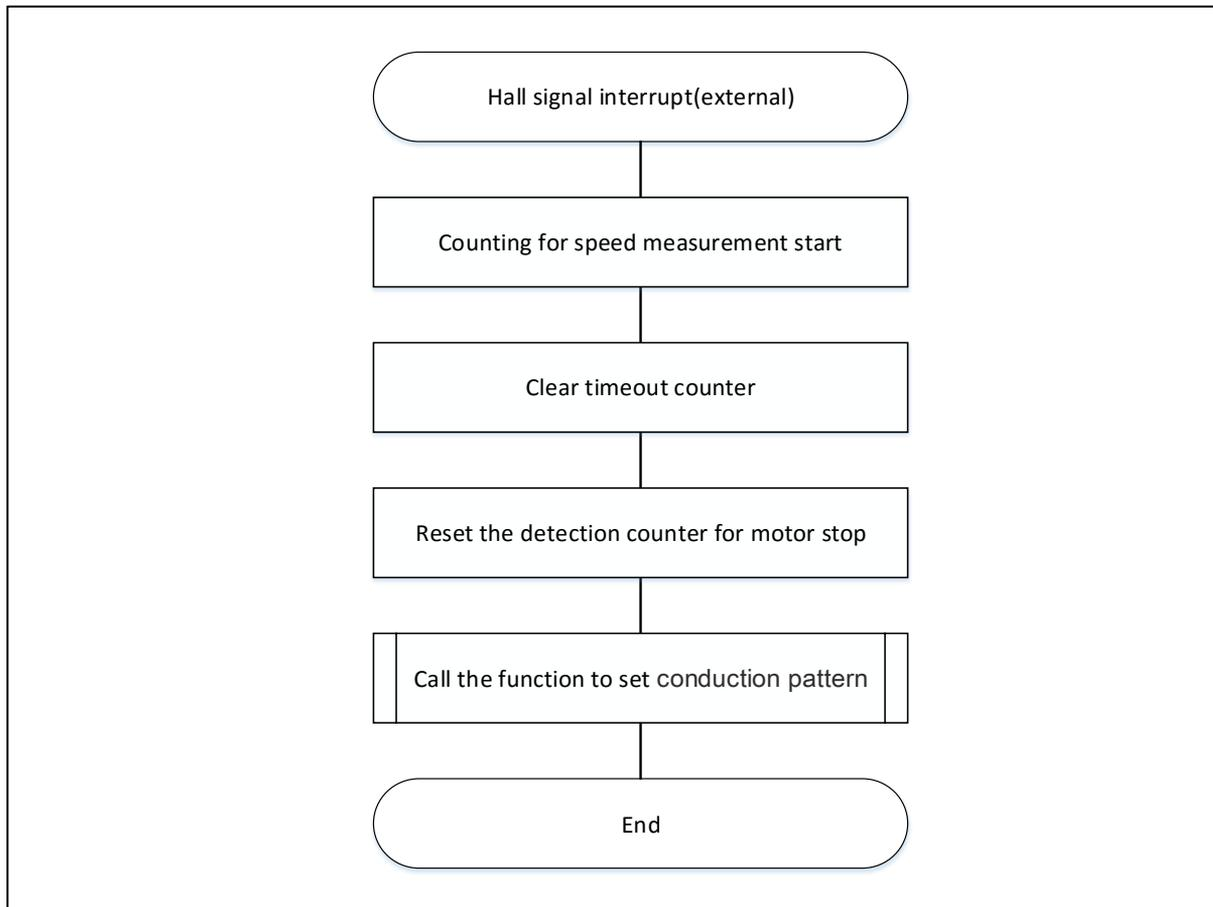
Figure 3-12 Hall signal Interrupt Handling (common process)
