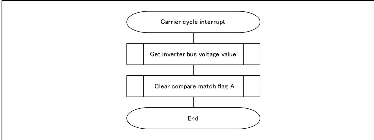
Figure 3-8 50[μs] Cycle Interrupt Handling (120-degree Control using Hall sensors)
