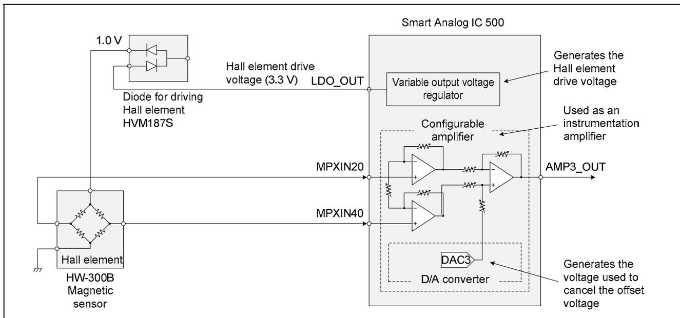
Figure 4-1 Example of Connecting Smart Analog IC 500 to the Hall Element
