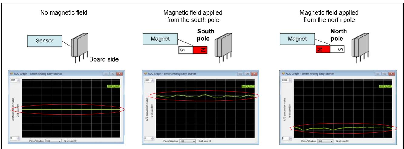
Figure 6-2 Operation Verification Waveforms
