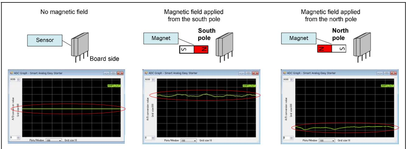
Figure 6-2 Operation Verification Waveforms
