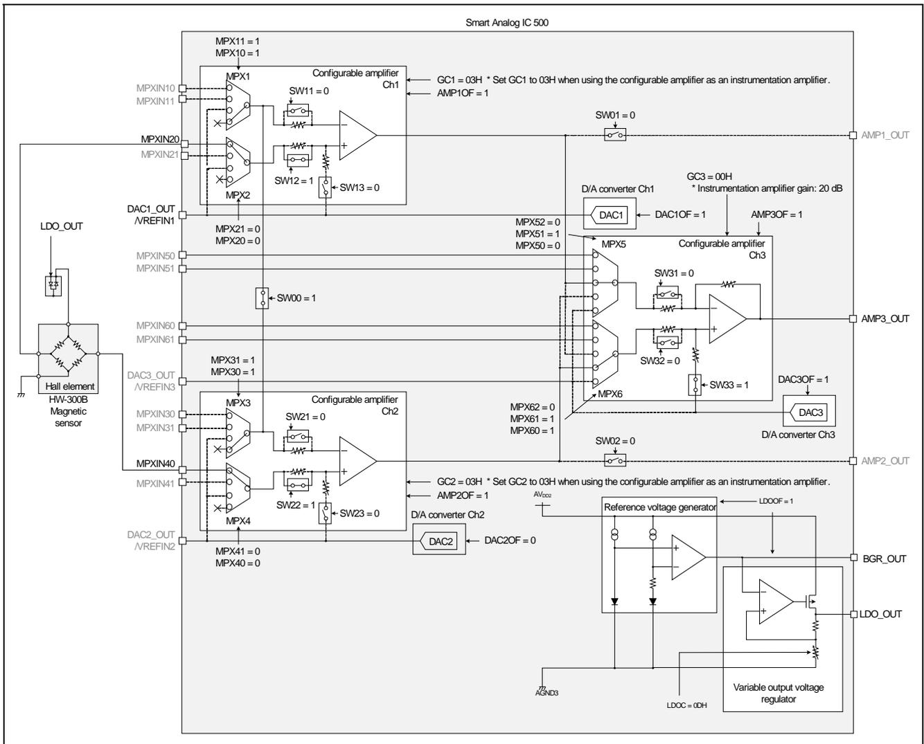
Figure 5-2 Circuit Configuration of Smart Analog IC 500
