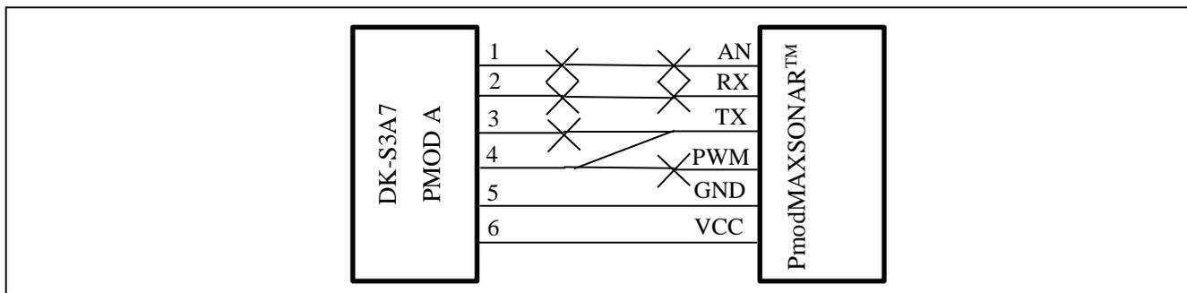
Figure 3 Connection diagram of DK-S3A7 and PmodMAXSONAR™
