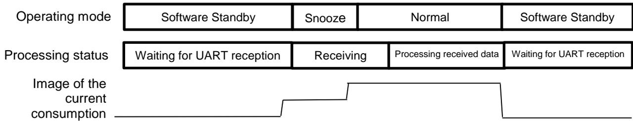
**Figure 4 Conceptual diagram of UART reception by Snooze mode**
