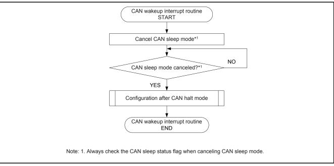
Figure 45 CAN Wakeup Procedure in CAN Halt Mode
