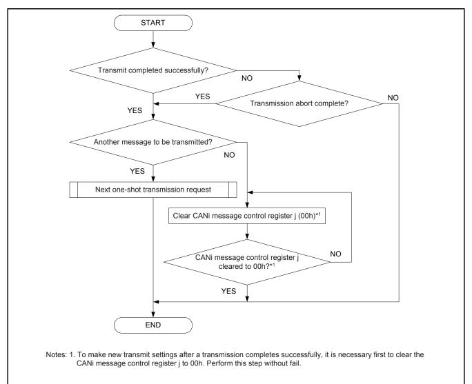
Figure 10 One-Shot Transmission Complete Procedure
