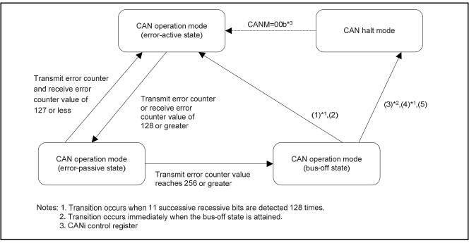
Figure 34 Transition to and from the Bus-Off State
