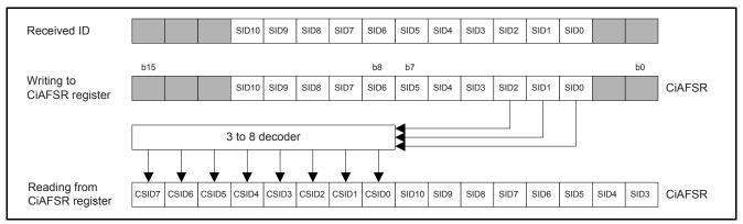
Figure 40 States when Writing to and Reading from CANi Acceptance Filter Support Register
