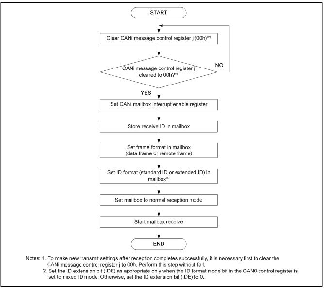
Figure 13 Normal Reception Request Procedure
