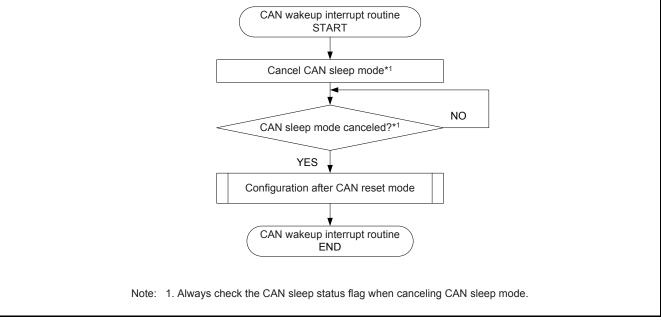
Figure 44 CAN Wakeup Procedure in CAN Reset Mode
