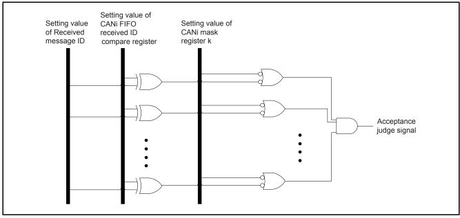
Figure 38 FIFO Receive ID Compare Register and Mask Register Configuration
