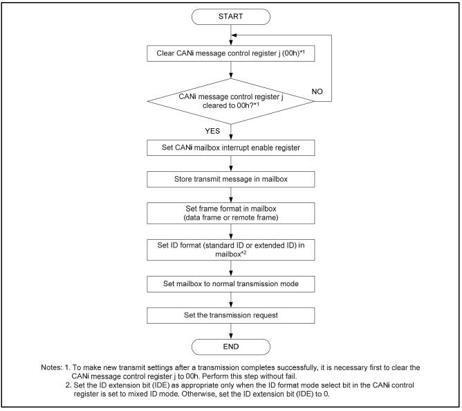
Figure 7 Normal Transmission Request Procedure
