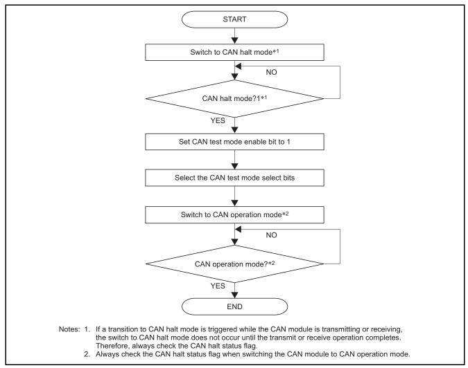
Figure 46 Test Mode Selection Procedure
