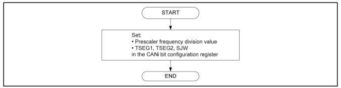
Figure 3 CAN Bit Timing and Transfer Speed Setting Procedure
