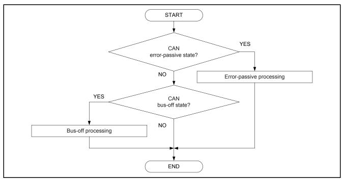
Figure 32 CAN Error State Checking Procedure (Using Polling)
