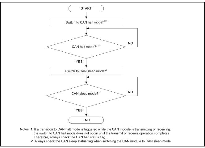
Figure 43 Procedure for Switching CAN Module to CAN Halt Mode and then CAN Sleep Mode
