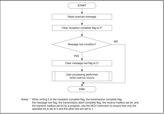
Figure 15 Message Reception Processing with Mailbox Set to Normal Reception Mode (Overrun Mode)
