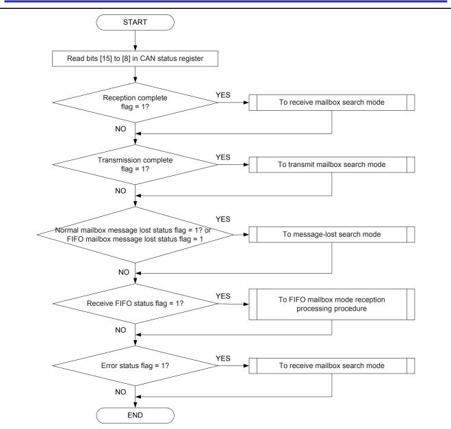
Figure 26 CAN Status Register Checking Example (Polling Operation)
