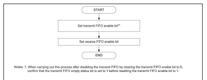
Figure 22 FIFO Mailbox Mode Setting Procedure in CAN Operation Mode
