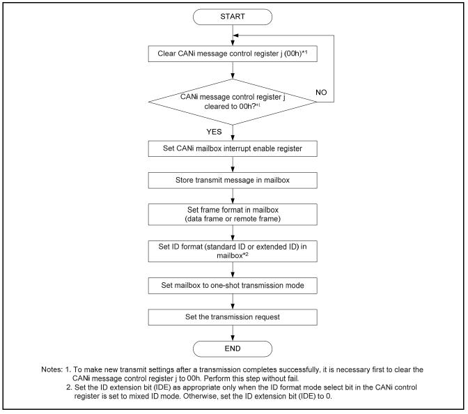
Figure 9 One-Shot Transmission Request Procedure
