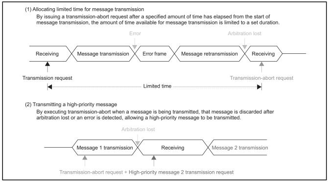
Figure 11 Transmission-Abort Function Application Examples
