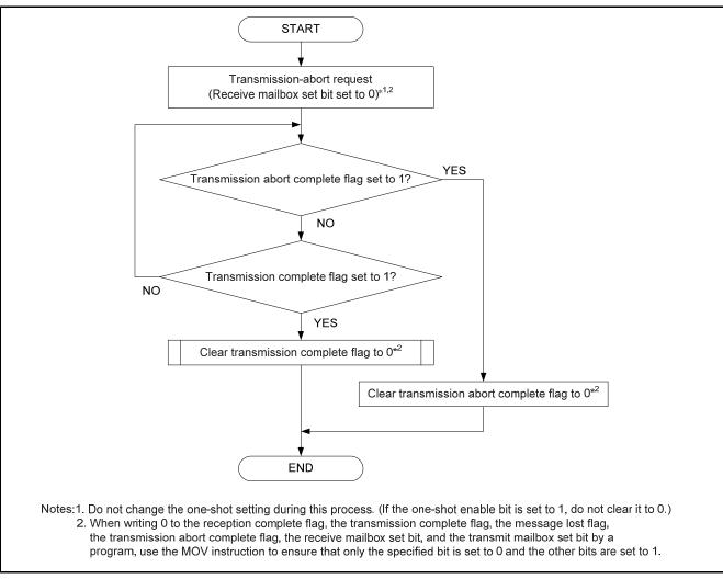
Figure 12 Transmission-Abort Procedure
