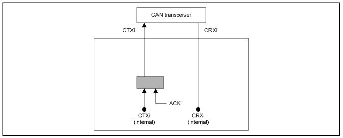
Figure 48 Self-Test Mode 0 Operation Illustration
