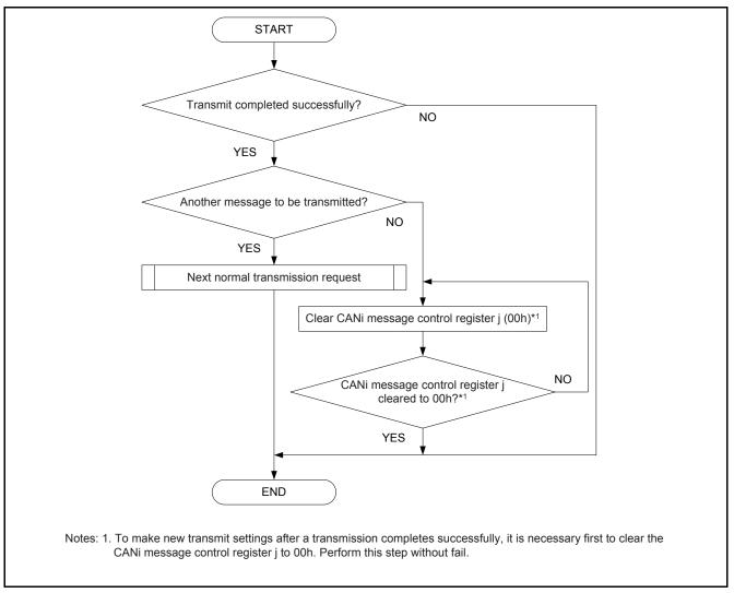
Figure 8 Normal Transmission Complete Procedure
