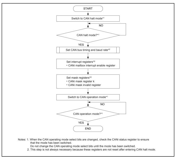
Figure 6 CAN Configuration Procedure after Transitioning to CAN Halt Mode
