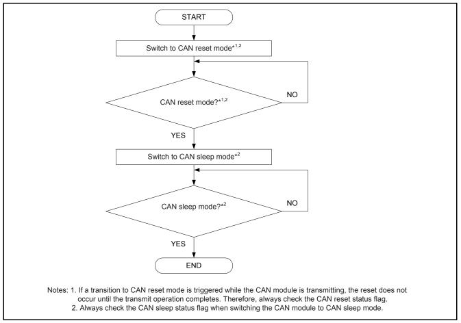
Figure 42 Procedure for Switching CAN Module to CAN Reset Mode and then CAN Sleep Mode
