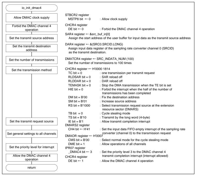
Figure 4.4 Initialization of DMAC channel 4
