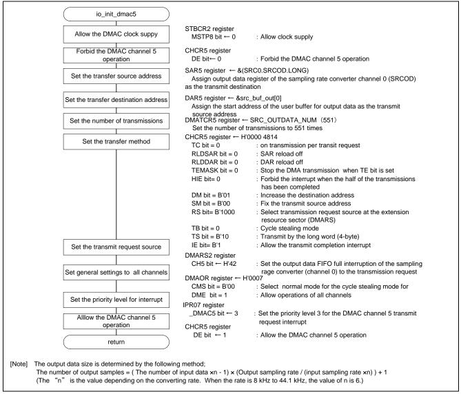
Figure 4.5 Initialization of DMAC channel 5
