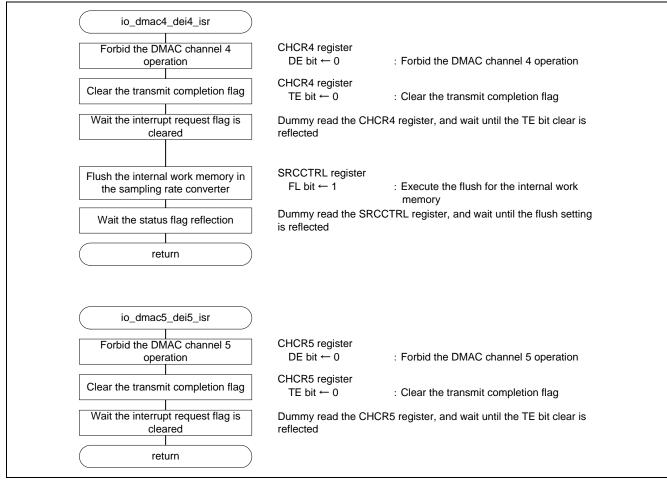
Figure 4.6 DMA transmit completion
