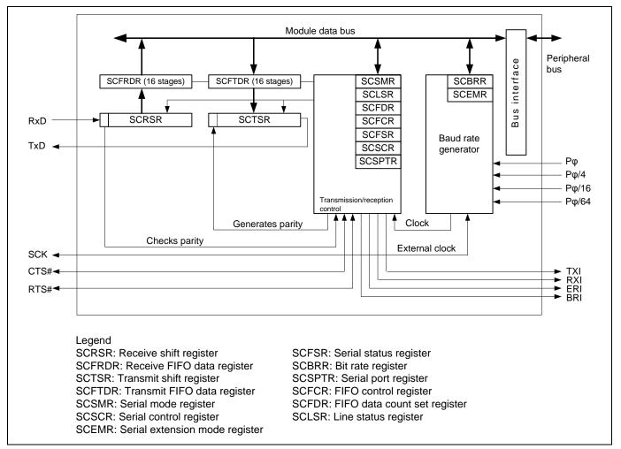
Figure 1 SCIF Block Diagram
