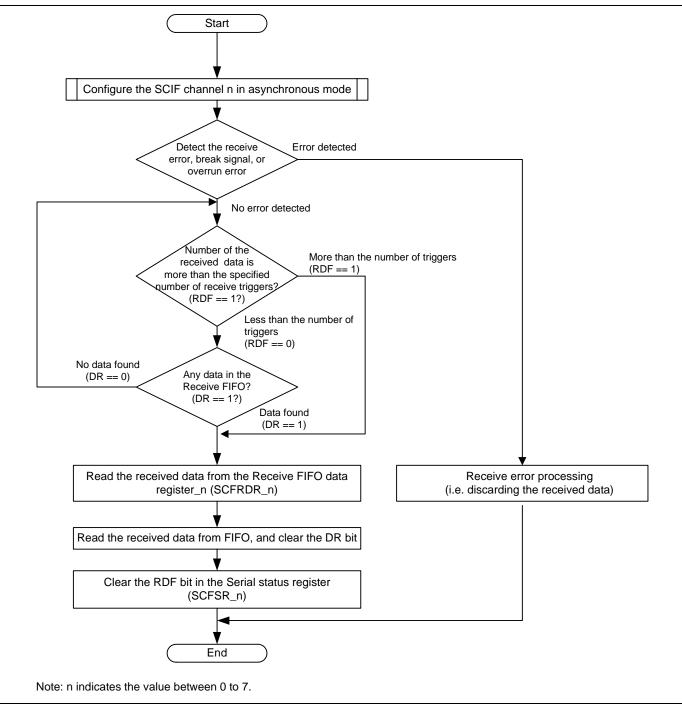
Figure 4 Flow Chart of the Reception in Asynchronous Mode
