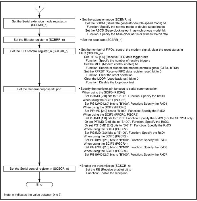
Figure 3 Flow Chart for Configuring the Reception in Asynchronous Mode (2/2)
