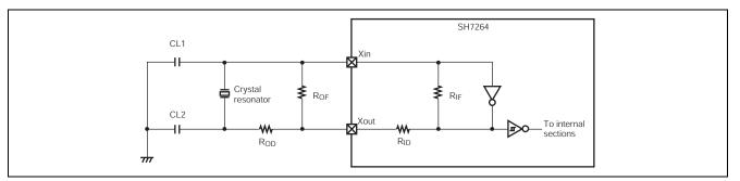
Figure 7 Connecting a Crystal Resonator
