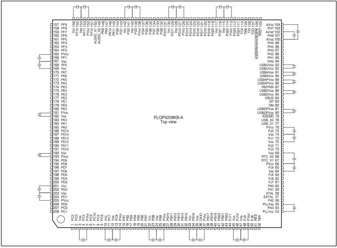
Figure 3 Installing an External Capacitor with the SH7264
