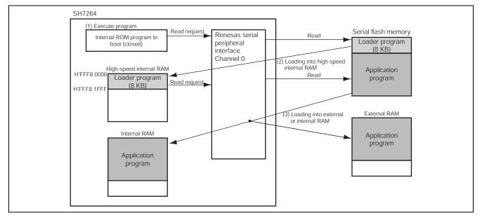
Figure 8 Boot Modes 1 and 3 Schematic View
