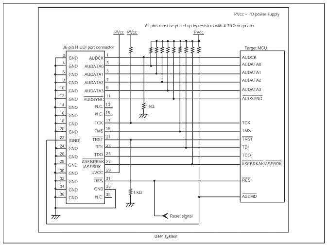
Figure 13 Recommended Circuit between the 36-pin H-UDI Port Connector and MCU (with E10A-USB)
