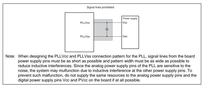
Figure 1 Note on Using PLL Oscillation Circuit
