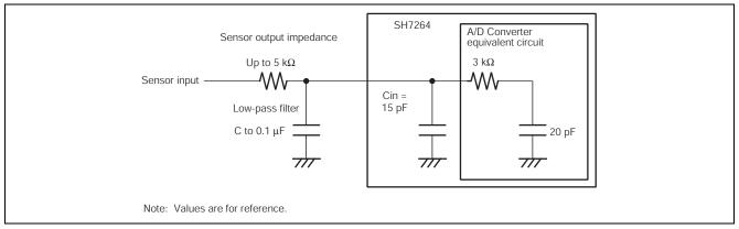
Figure 16 Analog Input Circuit Example
