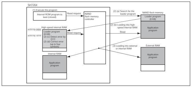
Figure 9 Boot Mode 2 Schematic View
