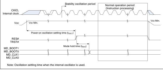
Figure 4 Relations between Power-on/off and Clock, Reset Signals
