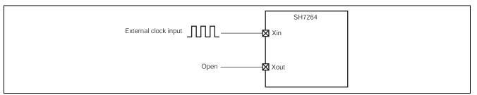
Figure 6 Connecting an External Clock
