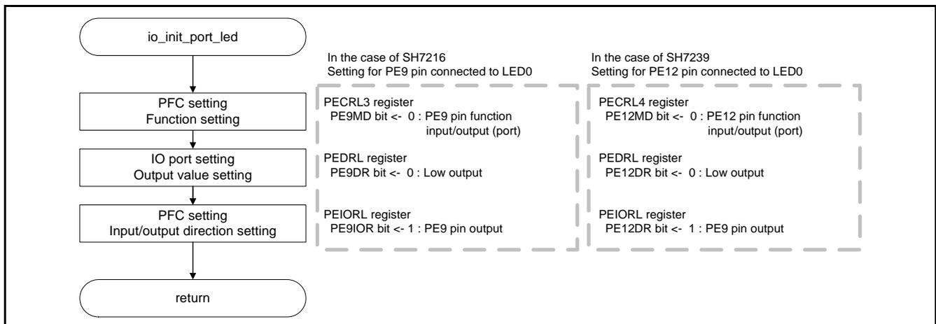
Figure 6.3 Initialization of IO Port for LED
