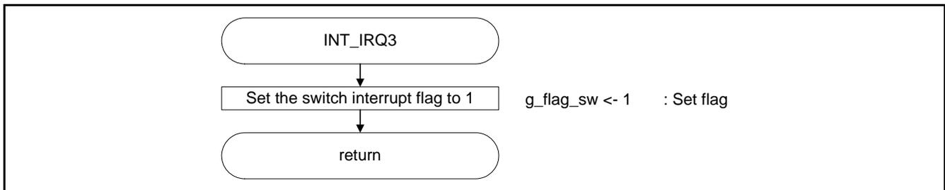
Figure 6.6 IRQ3 Interrupt Processing (SH7239)
