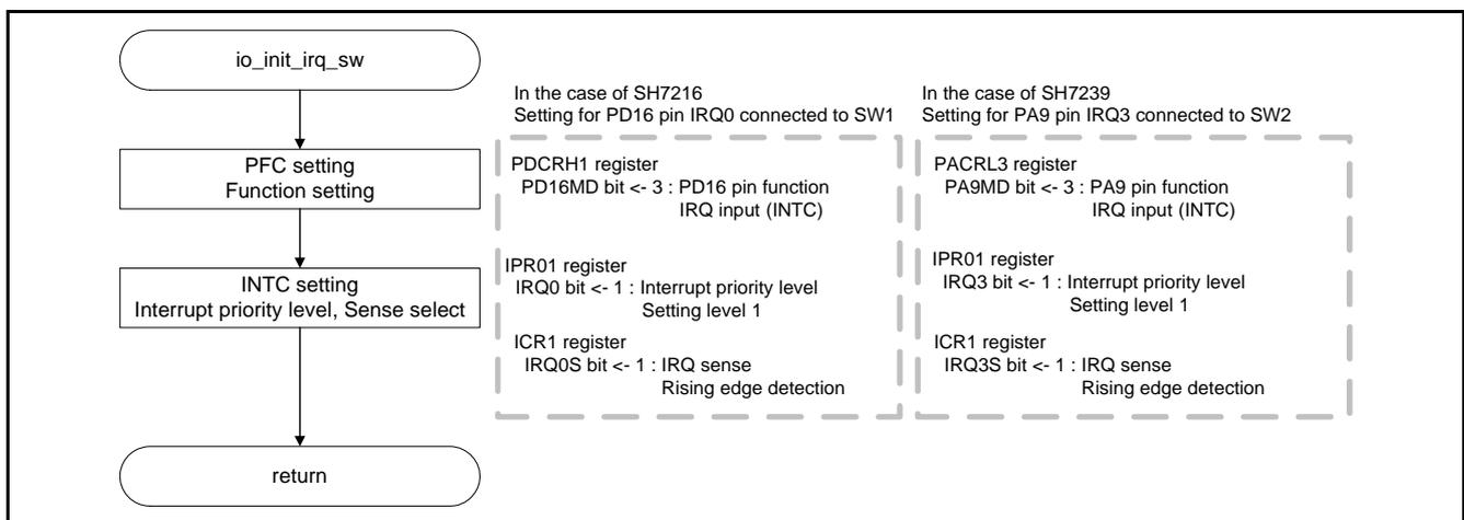
Figure 6.4 Initialization of IRQ Interrupt for the Switch
