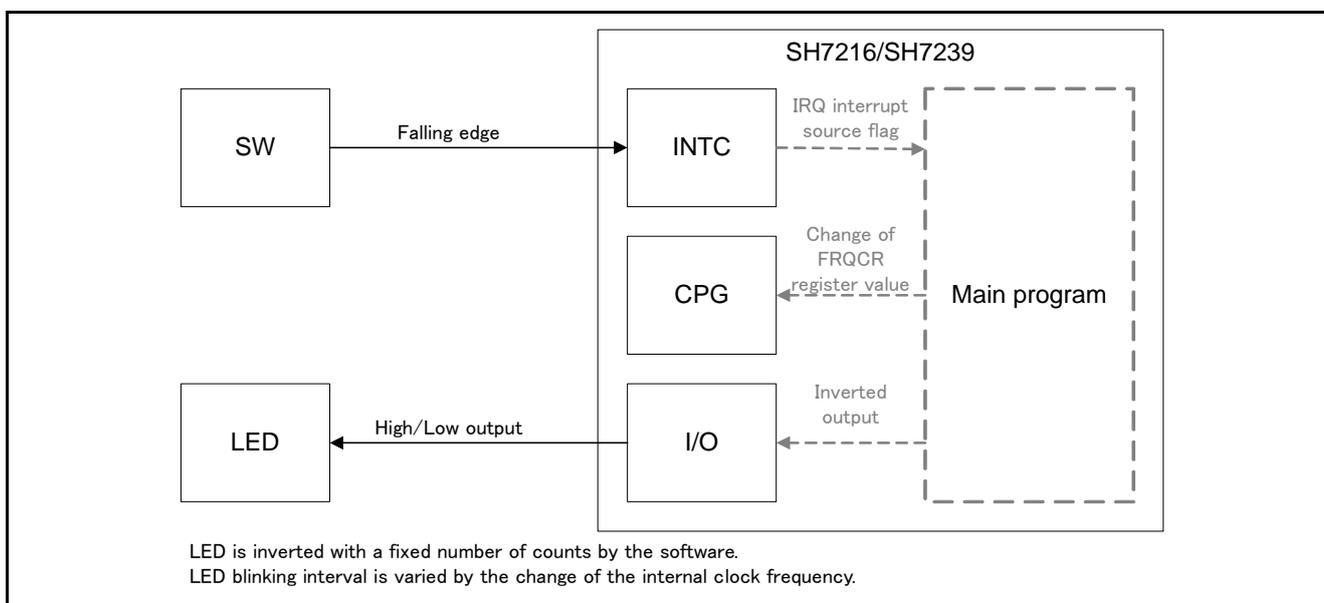
**Figure 1.1 System Diagram**
