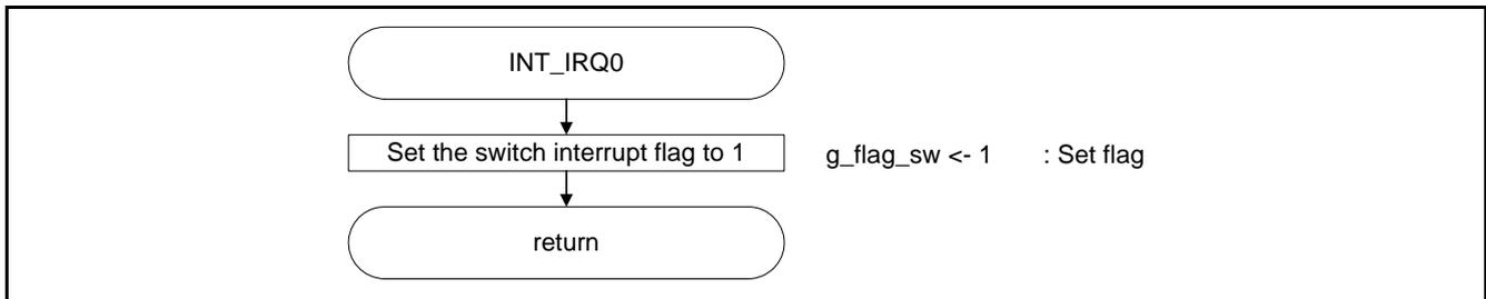
Figure 6.5 IRQ0 Interrupt Processing (SH7216)
