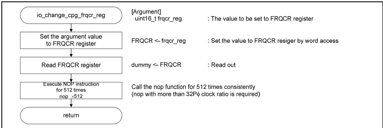
**Figure 6.9 Setting for FRQCR register**
