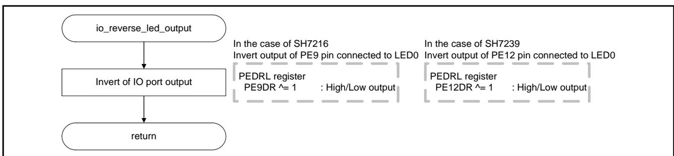
Figure 6.7 Inversion of LED Output
