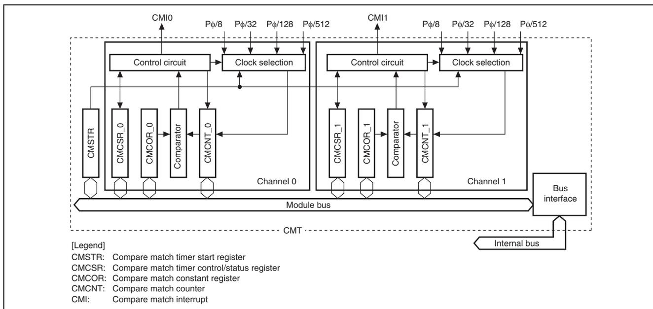
**Figure 1 CMT Block Diagram**
