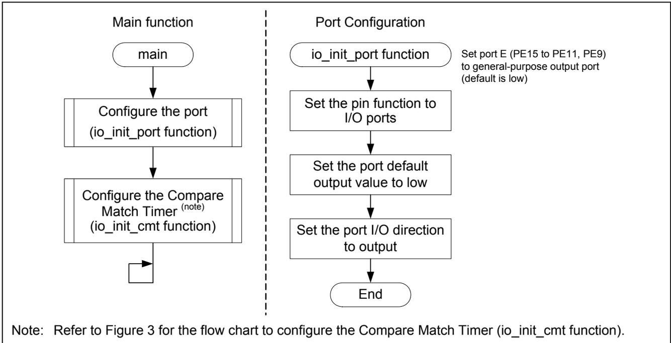
**Figure 5 Main Function and Port Configuration (io\_init\_port function) Flow Chart**
