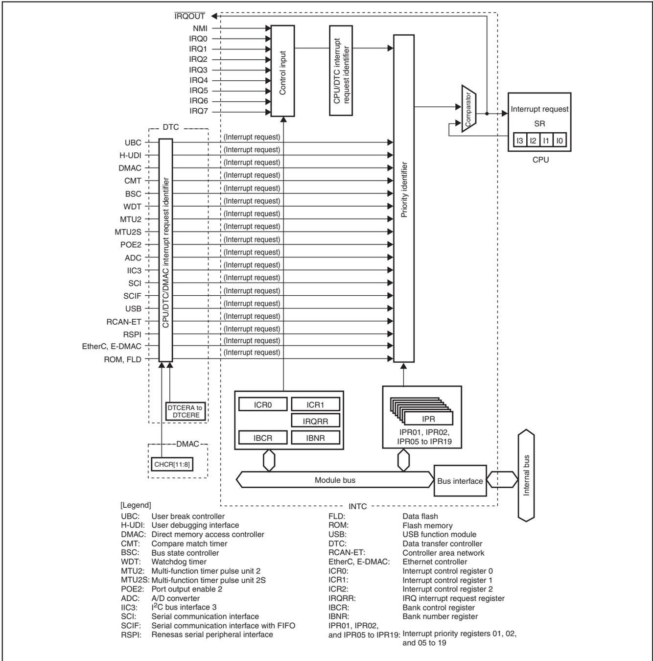
Figure 2 INTC Block Diagram
