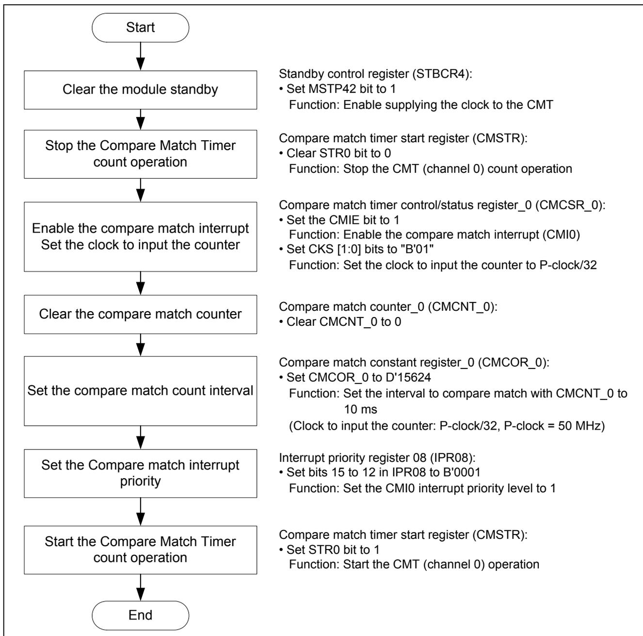
Figure 3 Flow Chart for Configuring the CMT Periodic Count Operation
