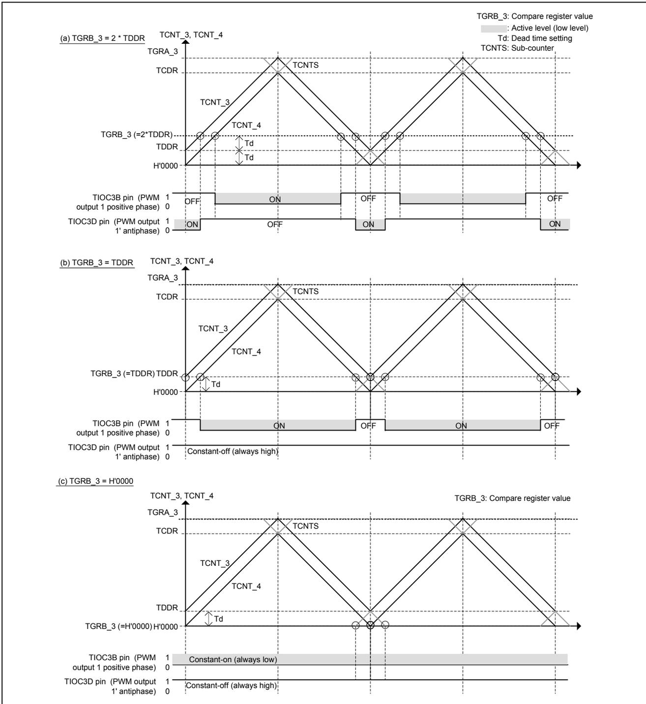
Figure 10 Examples of PWM Waveform Output (2)
