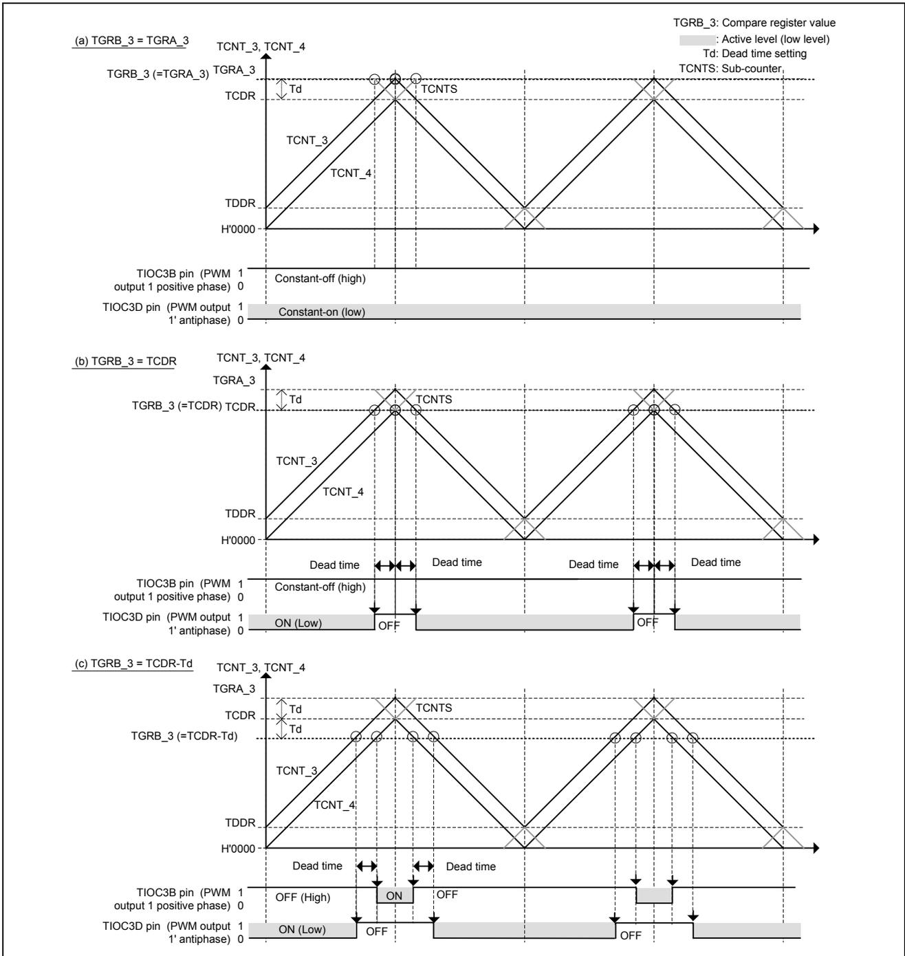
Figure 9 Examples of PWM Waveform Output (1)
