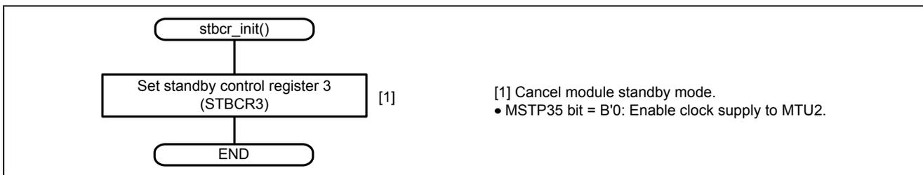
Figure 12 Initialization: Release from Standby
