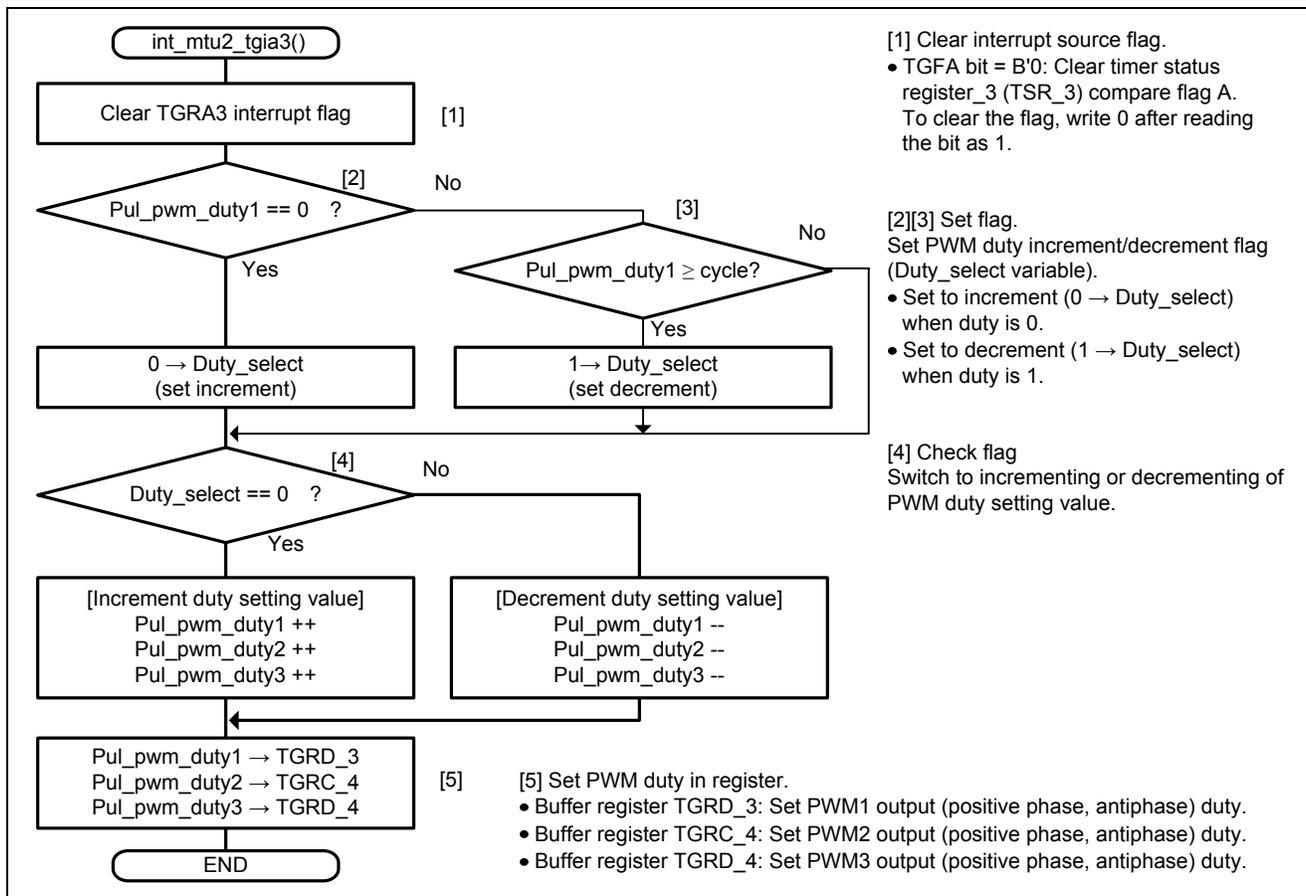
Figure 15 Interrupt Handling
