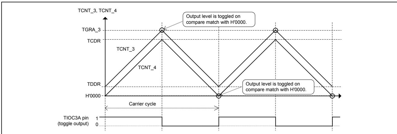
**Figure 8 Operation for Toggling an Output in Synchronization with the PWM Cycle**
