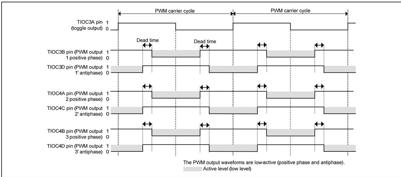
Figure 4 Output Waveforms in Complementary PWM Mode Operation
