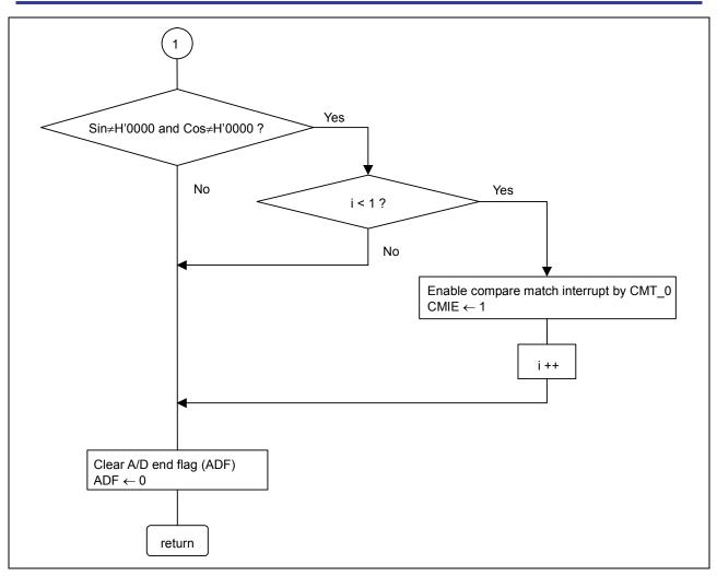
Figure 22 ADC\_0 Interrupt Process Flow (2)
