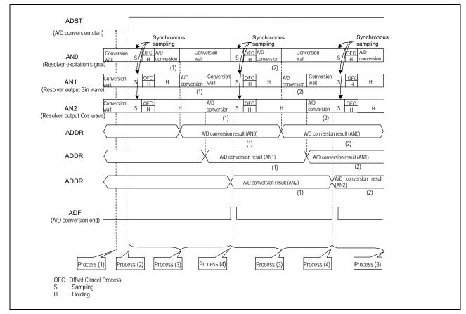
Figure 9 A/D Conversion Operation in Continuous Scan Mode
