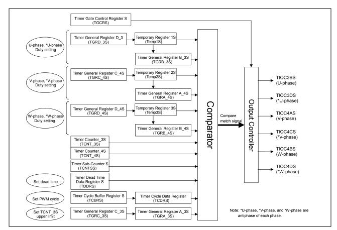
Figure 11 Block Diagram when in Complementary PWM Mode (Channel 3/4)
