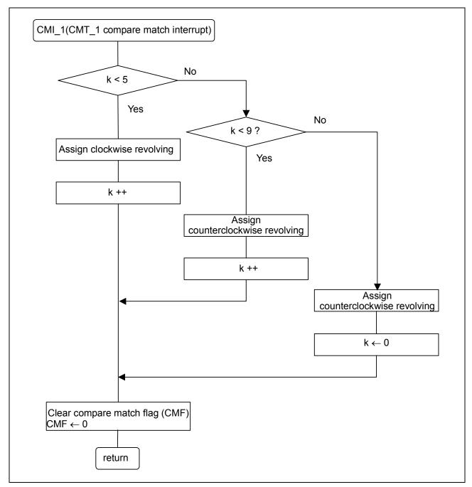
Figure 24 CMT\_1 Interrupt Process Flow
