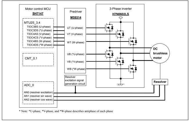
Figure1 Overview of Resolver Built-in DC Brushless Motor Control System
