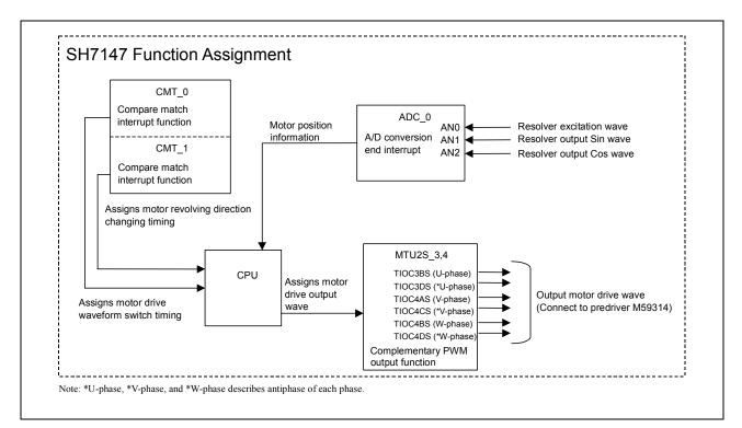
Figure 2 SH7147 Control Block Diagram
