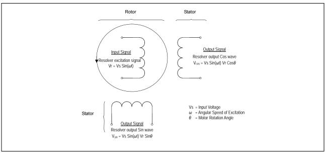
Figure 4 Diagram of Resolver Principle
