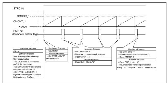
Figure 15 Principle of CMT\_1 Operation (Assign motor revolving direction reversing timing)
