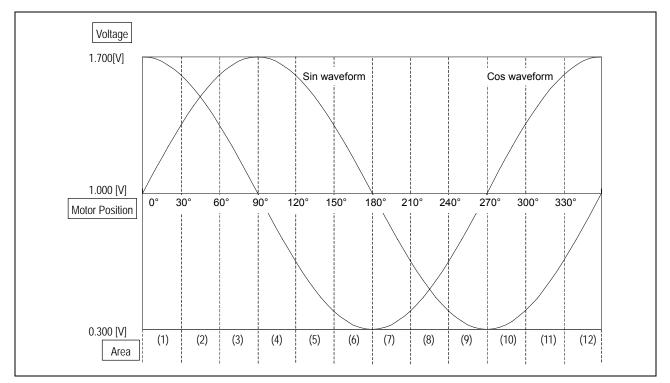
Figure 7 Motor Position and Sin Waveform/ Cos Waveform
