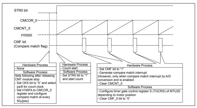
Figure 14 Principle of CMT\_0 Operation (Assign TGCRS setting timing)
