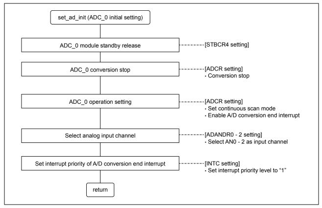
Figure 18 ADC\_0 Initial Setting Flow
