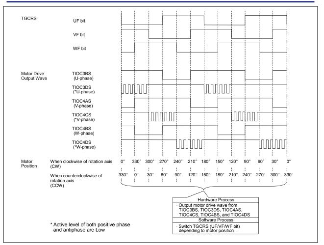
Figure 10 Motor Drive Wave by TGCRS (UF, VF, WF bit) Switch
