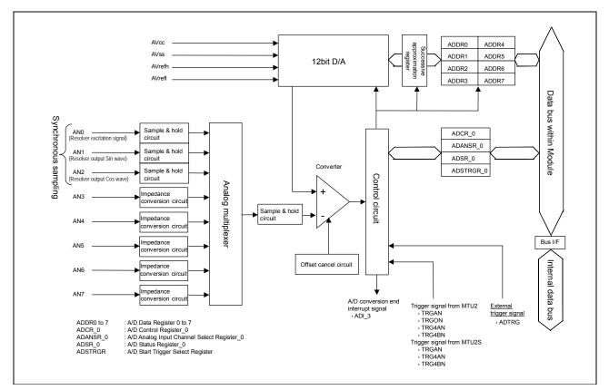
Figure 3 ADC\_0 Block Diagram
