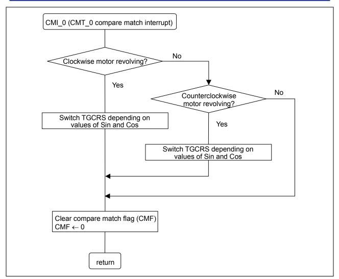
Figure 23 CMT\_0 Interrupt Process Flow
