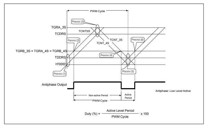
Figure 12 Counter Operation and Duty/PWM Cycle
