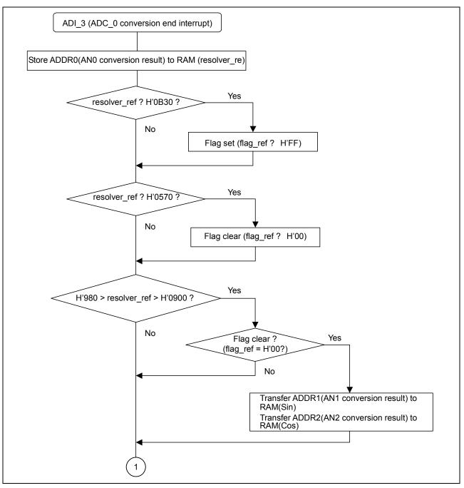
Figure 21 ADC\_0 Interrupt Process Flow (1)
