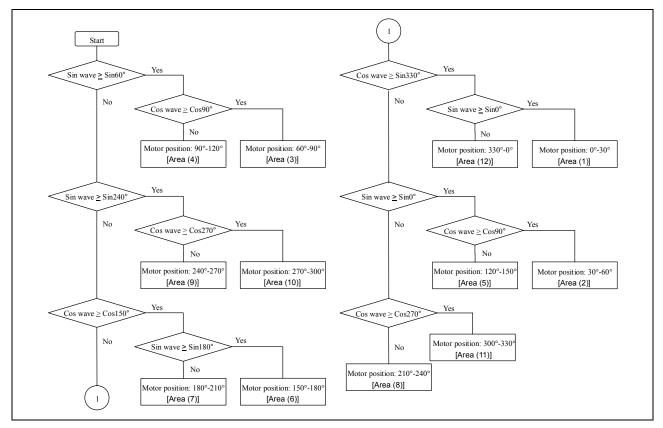
Figure 8 Motor Position Determining Flow
