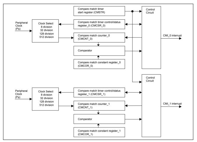
Figure 13 CMT Block Diagram
