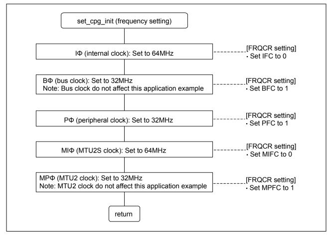
Figure 17 Frequency Setting Process Flow
