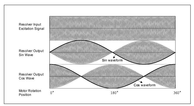
Figure 5 Resolver Input/Output Signal and Sin wave/ Cos wave (per motor revolution)
