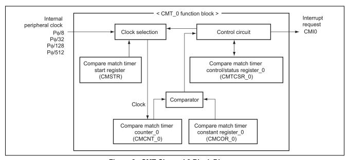
Figure 3 CMT Channel 0 Block Diagram
