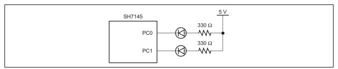
Figure 1 Connections between SH7145F and LEDs
