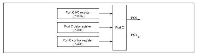
Figure 4 Port C Block Diagram
