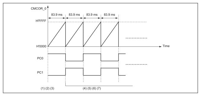
Figure 5 CMT Interrupt and Port Outputs
