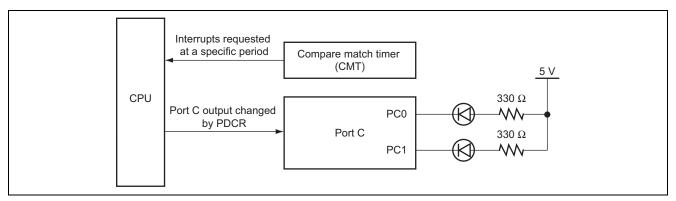
Figure 2 Function Block Diagram
