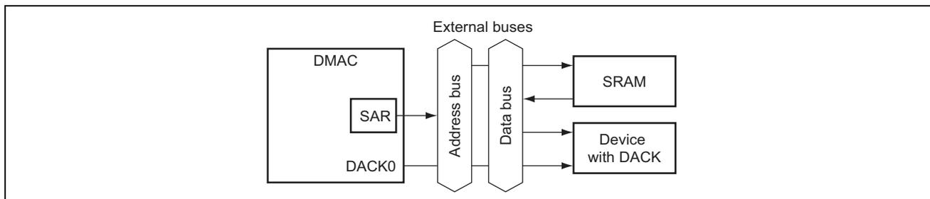
**Figure 1 Data Transfer Using DMAC**
