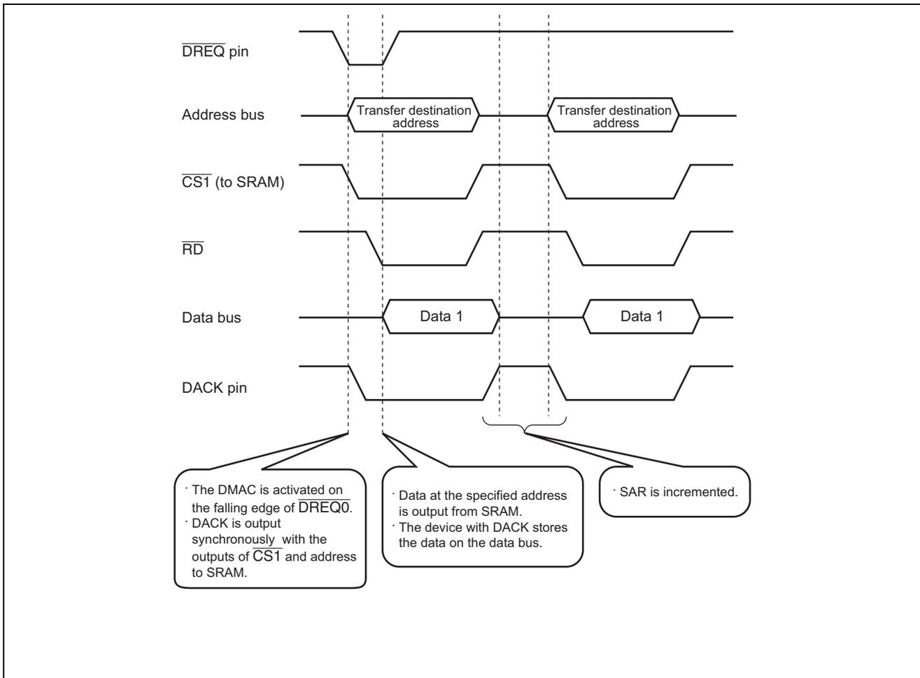
Figure 3 Operation in Single Address Mode
