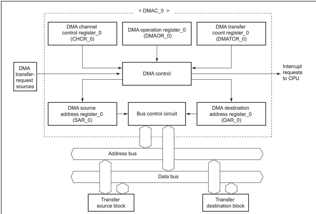
Figure 2 DMAC Block Diagram (ch0)
